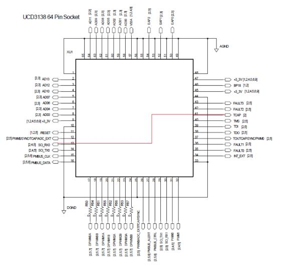
Figure 1. UCD3138 Pin Configuration[1]
