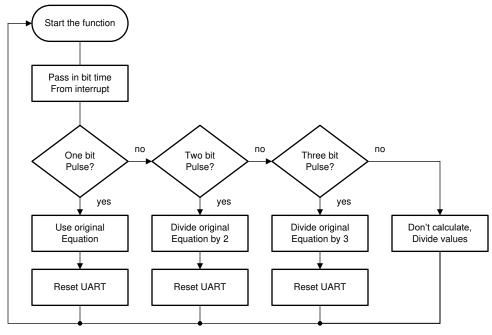
Figure 5. Flowchart of Baud Rate Configuration
