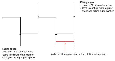
Figure 2. Timer Capture on a Waveform
