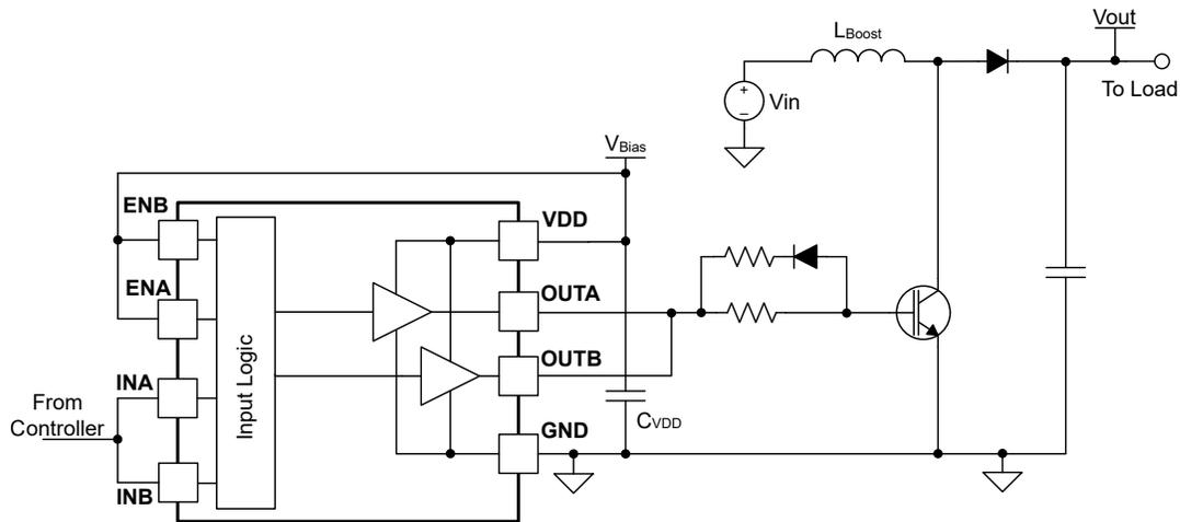
Figure 7-3. UCC27624 Used to Drive IGBT in the Boost Converter
