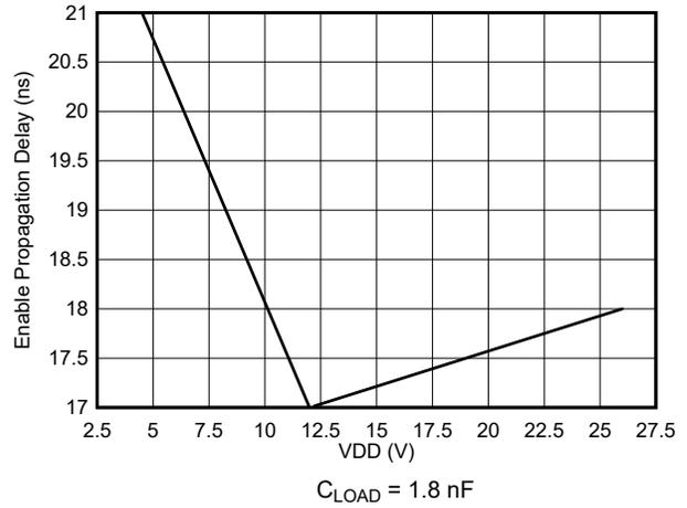
Figure 5-20. Enable to Output Rising Propagation Delay
