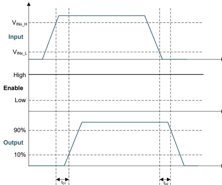
**Figure 5-2. Input-Output Operation**
