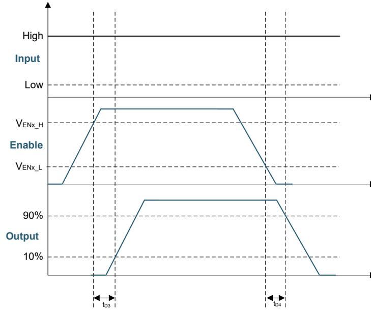
**Figure 5-1. Enable Function**
