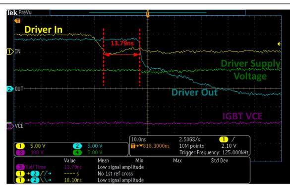
Vin = 210 V, Vout = 235 V, Iout = 1.14 A, Fsw = 100 kHz, driver supply voltage = 15 V, gate resistor = 0 Ω
