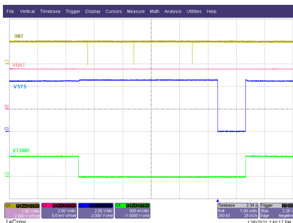
Figure 9-15. Wake1 Interrupt with VIN Present
