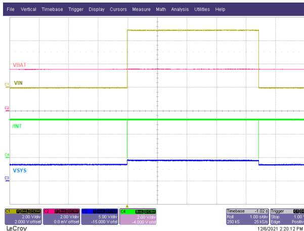
Figure 9-11. Power Good Interrupt on /INT
