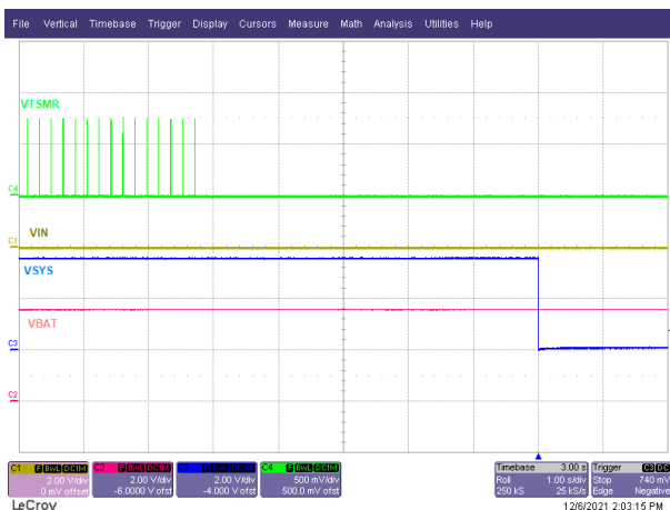
Figure 9-10. Shipmode Entry on VIN Removal
