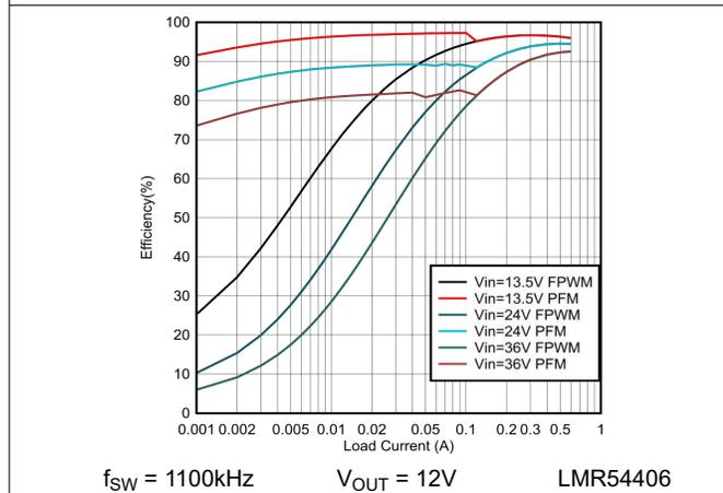
Figure 6-5. 12V Efficiency Versus Load Current
