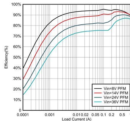
Efficiency Versus Output Current;
