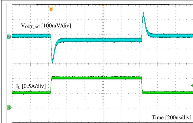
Figure 8-7. Load Transient
