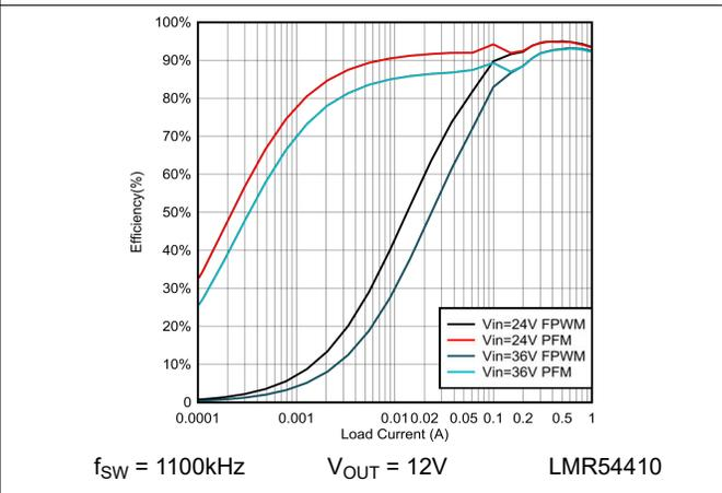
Figure 6-6. 12V Efficiency Versus Load Current
