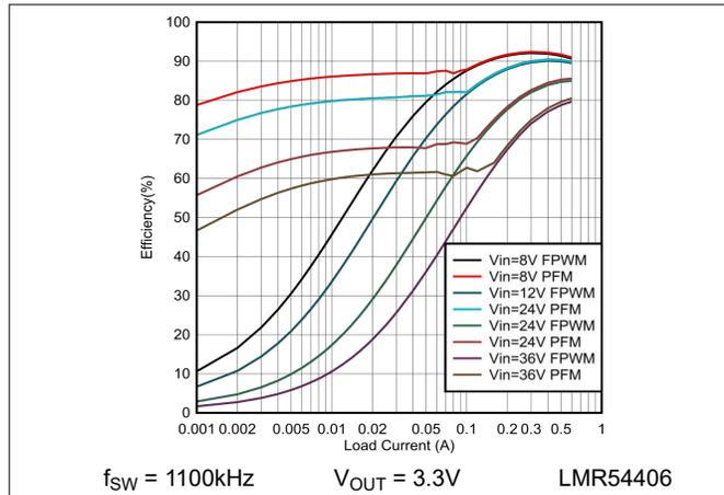
Figure 6-1. 3.3V Efficiency Versus Load Current
