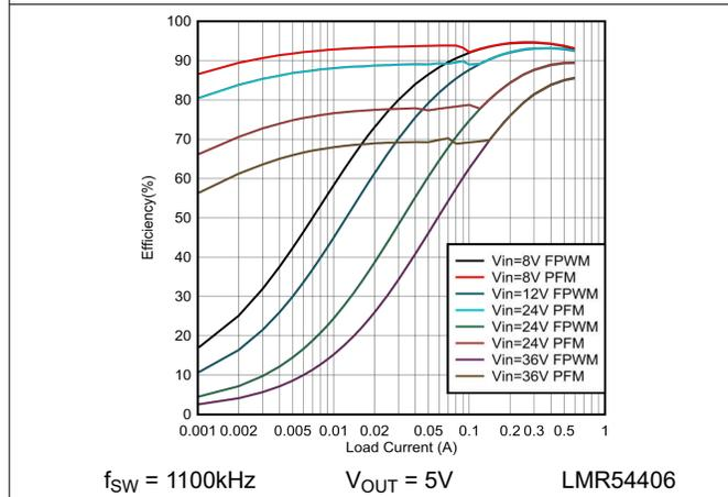
Figure 6-3. 5V Efficiency Versus Load Current
