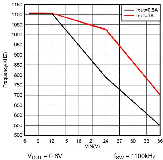
Figure 7-4. Frequency Foldback at  $T_{ON\_MIN}$
