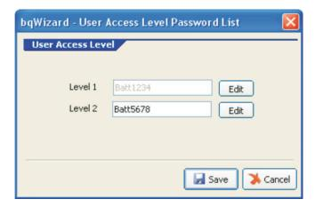
The bqWizard<sup>™</sup> software can only be operated at Level 2 access. Without a Level 2 password, the GUI starts as normal. If a Level 2 password is programmed, then the GUI always prompts the user to enter the password on startup to unseal the device.
