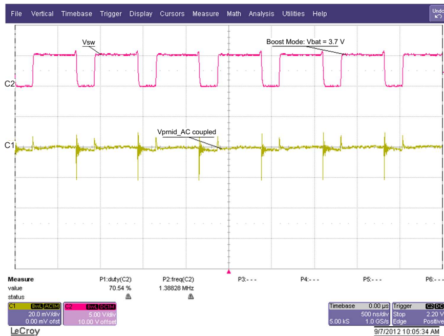
Figure 5. Boost Mode Ripple and Duty Cycle; V_{BAT} = 3.7\text{ V}
