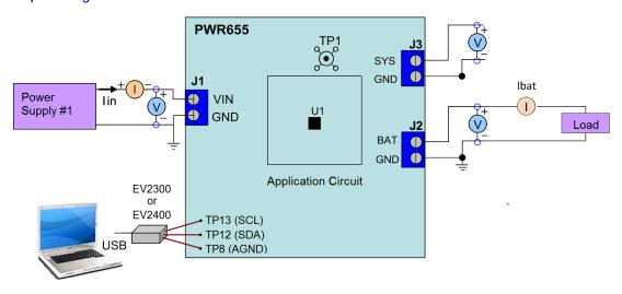
Figure 2. Original Test Setup for PWR655
