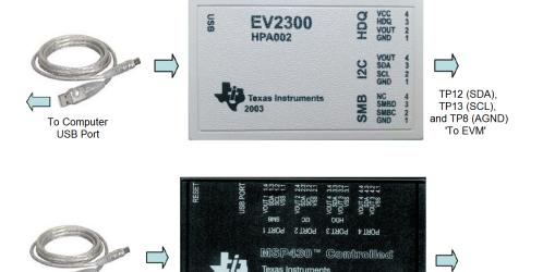
Figure 1. Connections of the EV2300 or EV2400 Kit
