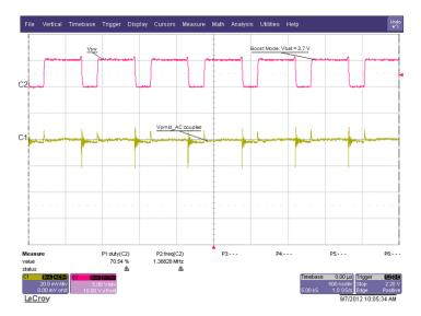
Figure 6. Boost Mode Ripple and Duty Cycle:  $V_{BAT} = 3.7 \text{ V}$
