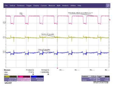
Figure 5. CHG Mode Ripple and Duty Cycle:  $V_{BUS} = 5 \text{ V}$ ,  $V_{BAT} = 3.7 \text{ V}$
