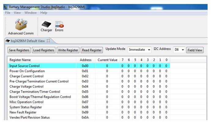
Figure 3. Main Window of the bq24296M Evaluation Software
