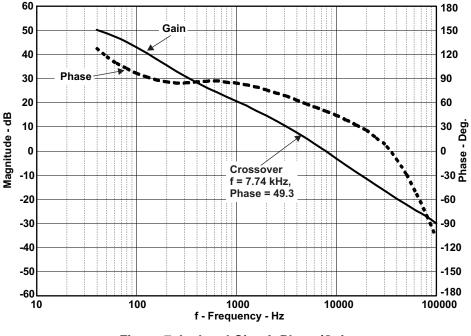
Figure 7. Isolated Circuit Phase/Gain
