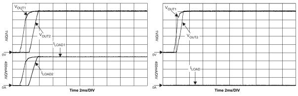
Figure 14. Isolated vs Non-isolated Circuit Startup
