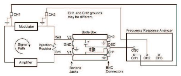
Figure 5. Set up for the Power Stage Phase/Gain Measurement Using the Venable Windows Software 4.0 For MODEL 3120, Venable Instruments®, 2006
