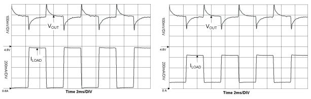
Figure 2. Isolated Circuit Transient Response
