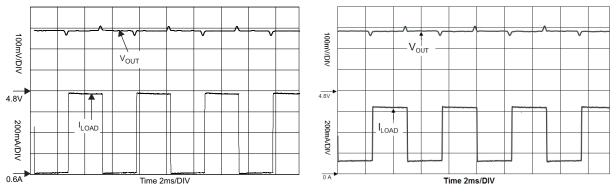
Figure 10. Non-isolated Circuit Transient Response
