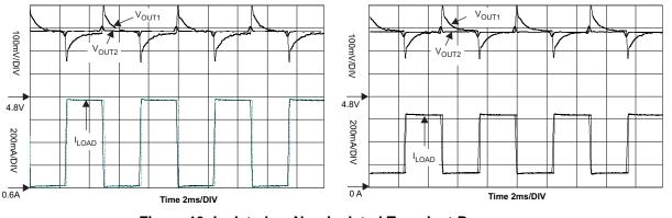
Figure 13. Isolated vs Non-isolated Transient Response
