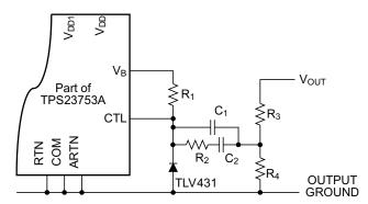
Figure 8. TL431 Error Amplifier Direct Interface
