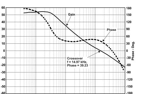
f - Frequency - Hz Figure 12. Non-isolated Circuit Phase/Gain
