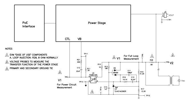
Figure 6. Setup for EVM Phase/Gain Measurement
