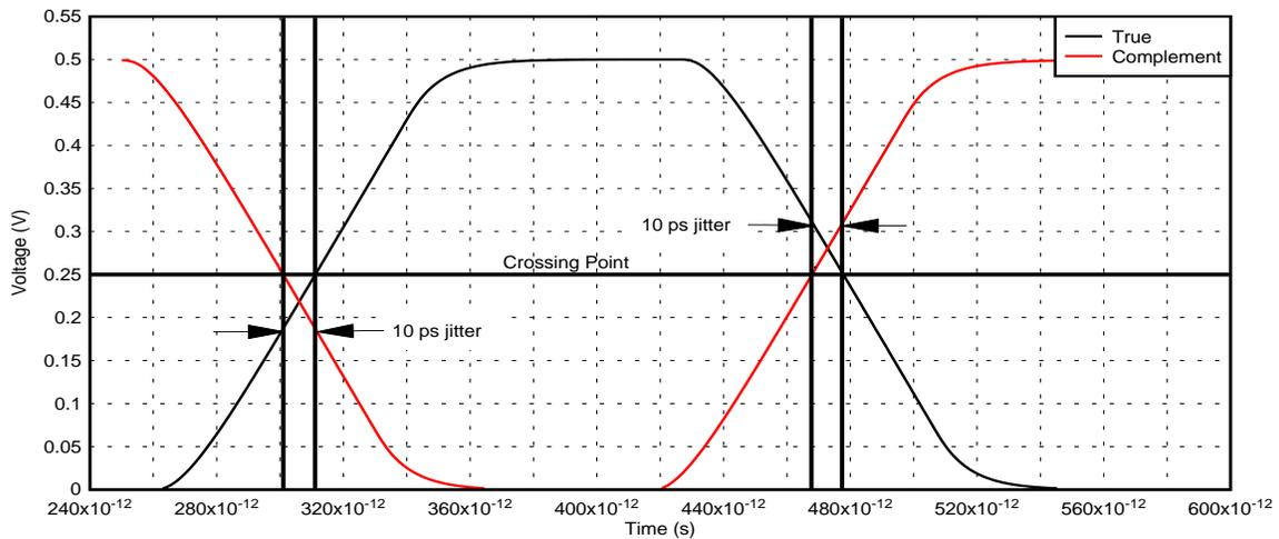
Figure 4. Jitter from Different Propagation Delays Within a TMD5 Pair
