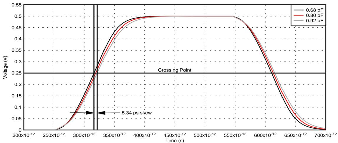
**Figure 3. Skew Added by  $t_r$  and Phase Delay Change From a 15% Capacitance Variation**
