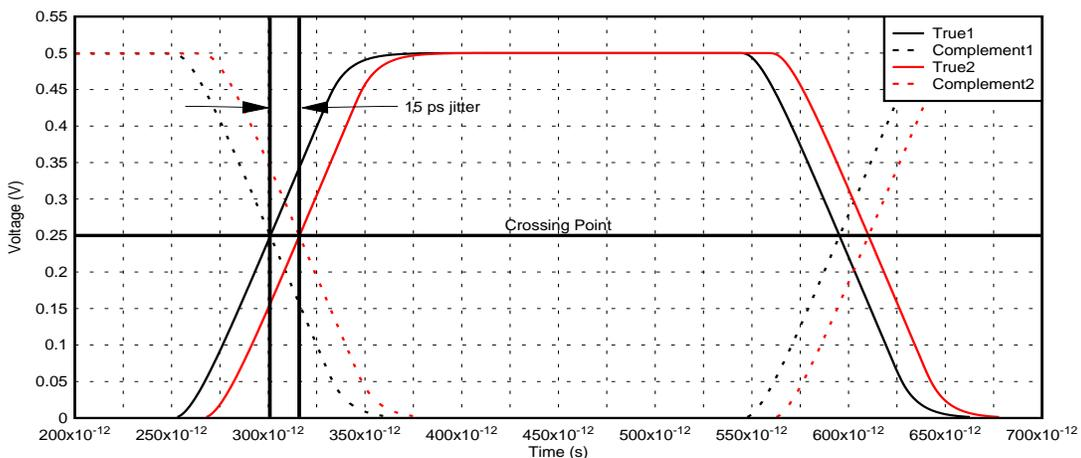
Figure 2. Inter-Pair Skew From Different Electrical Lengths
