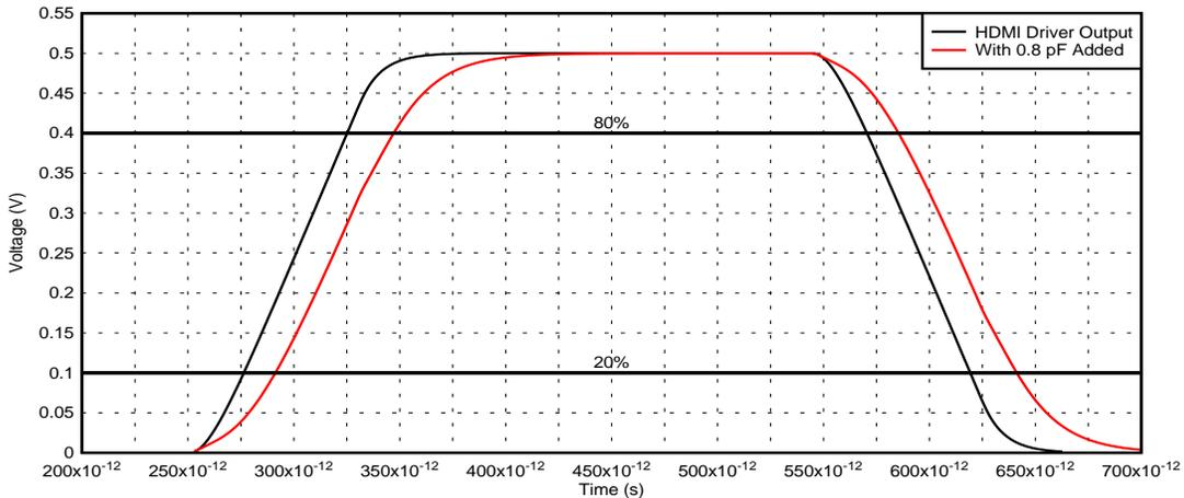
Figure 1. Change in  $t_r$  and  $t_f$  by a Capacitive Load
