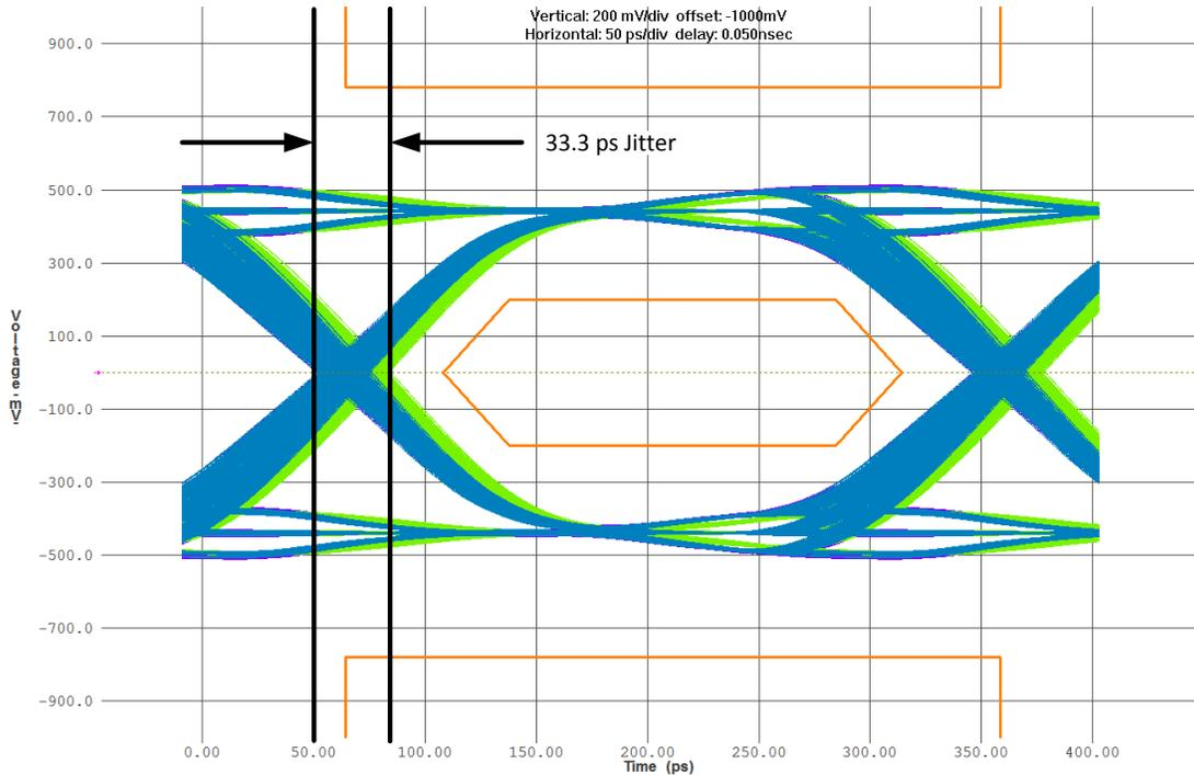
Figure 6. Three TMDS Data Eye Diagrams Combined
