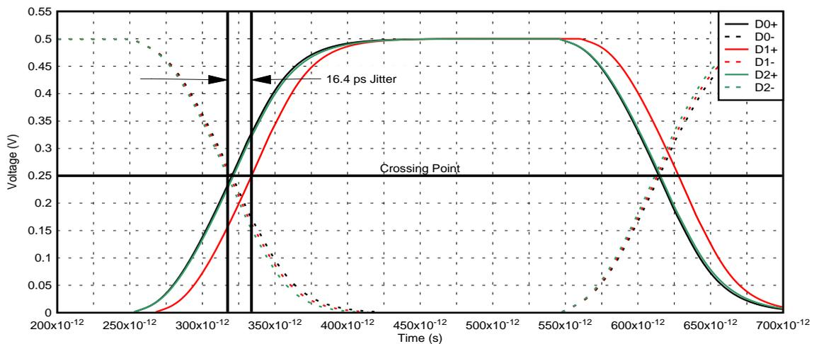
Figure 5. Data TMD5 Signals with Previous Skews Combined
