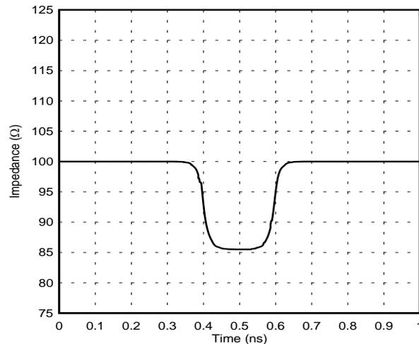
**Figure 7. 192 ps  $t_r$  TDR of 0.6 pF Capacitance**
