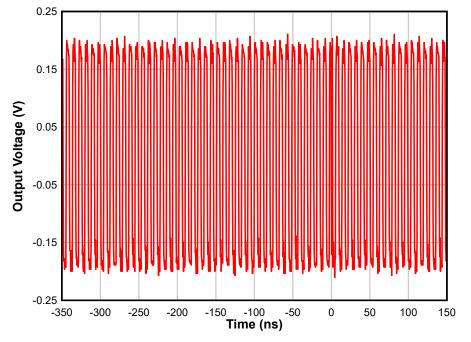
Figure 3-5. Example of an SEU That Lasted 1 Clock Cycle From Ion Run #36, with an LETeff of 70 MeV-cm<sup>2</sup>/mg and the DUT in Dual Loop Mode
