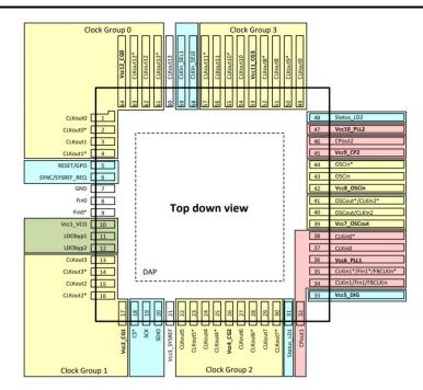
Figure 1-3. LMK04832-SP Pinout
