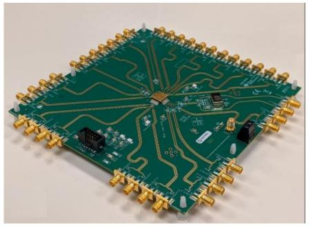
Figure 2-1. LMK04832EVM-CVAL Evaluation Board
