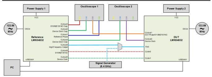
Figure 2-2. Block Diagram of Test Setup
