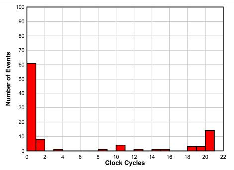
Figure 3-9. Histogram of the Length of Events in Clock Cycles for Ion Run #28 at an LETeff of 48 MeV-cm<sup>2</sup>/mg and the DUT in Single Loop 0-Delay Mode. There Were a Total of 98 Events in This Ion Run.
