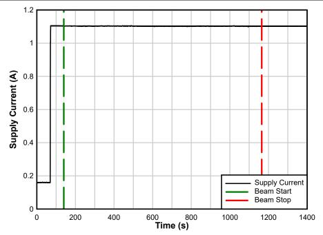
Figure 3-3. Supply Current for Ion Run #3 with DUT in Single Loop, 0-Delay Mode, LETeff at 121 MeVcm<sup>2</sup>/mg and DUT Board Thermister Reading of 125°C
