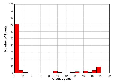
Figure 3-10. Histogram of the Length of Events in Clock Cycles for Ion Run #34 at an LETeff of 70 MeV-cm<sup>2</sup>/mg and the DUT in Dual Loop Mode. There Were a Total of 100 Events in This Ion Run.
