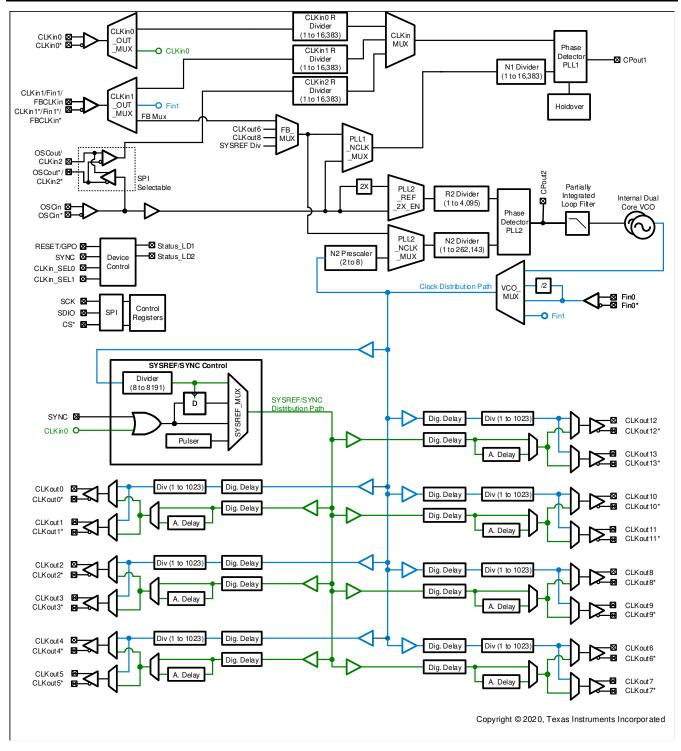
Figure 1-2. LMK04832-SP Detailed Block Diagram
