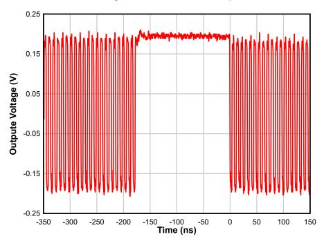
Figure 3-6. Example of an SEU that Lasted Multiple Clock Cycles From Ion Run #36, with an LETeff of 70 MeV-cm<sup>2</sup>/mg and the DUT in Dual Loop Mode
