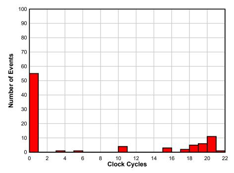
Figure 3-8. Histogram of the Length of Events in Clock Cycles for Ion Run #27 at an LETeff of 29.5 MeV-cm<sup>2</sup>/mg and the DUT in Dual Loop, Nested, 0-Delay Mode. There Were a Total of 89 Events in this Ion Run.
