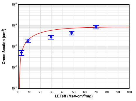
Figure 3-11. SEU Cross Section vs. LETeff for Dual Loop Mode with a Weibull Plot Fitted to the Data
