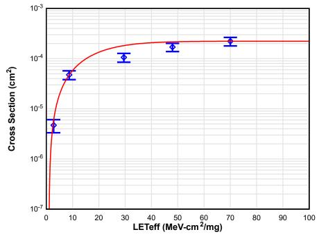
Figure 3-14. SEU Cross Section vs. LETeff for Distribution Mode with a Weibull Plot Fitted to the Data
