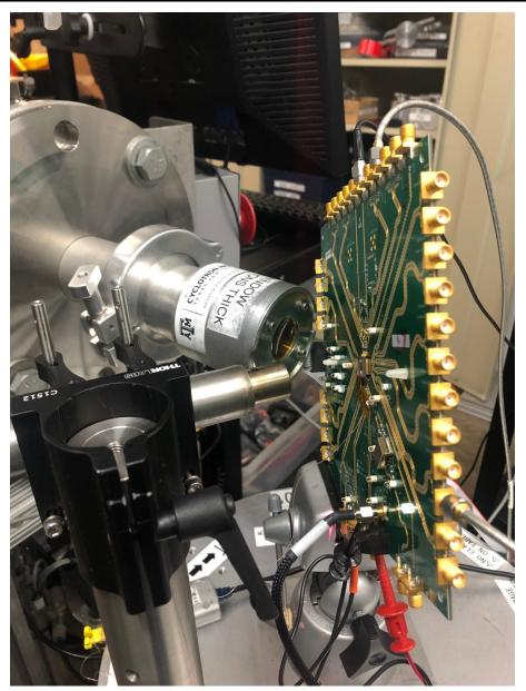
Figure 2-3. DUT Board Set Up with Heat Gun for SEL Testing at TAMU. The Board is Positioned So the DUT Will Have a 44° Incident Angle to the Ion Beam.
