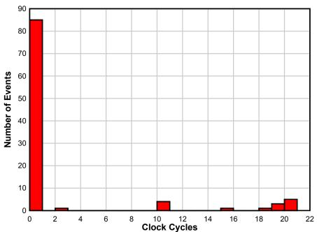
Figure 3-7. Histogram of the Length of Events in Clock Cycles for Ion Run #18 at an LETeff of 8.7 MeV-cm<sup>2</sup>/mg and the DUT in Distribution Mode. There Were a Total of 100 Events in This Ion Run.
