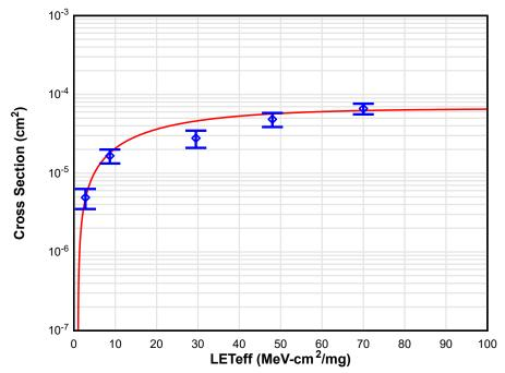
Figure 3-13. SEU Cross Section vs. LETeff for Single Loop Mode with a Weibull Plot Fitted to the Data
