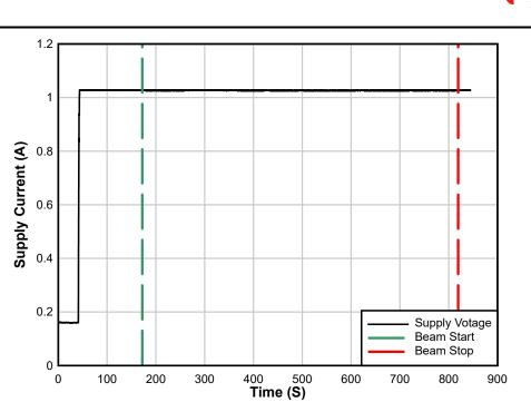
Figure 3-1. Supply Current for Ion Run #1 with DUT in Dual Loop Mode, LETeff at 121 MeV-cm<sup>2</sup>/mg and DUT Board Thermister Reading of 133°C
