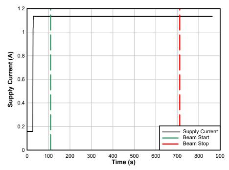
Figure 3-2. Supply Current for Ion Run #2 with DUT in Dual Loop, Holdover Mode, LETeff at 121 MeVcm<sup>2</sup>/mg and DUT Board Thermister Reading of 126°C
