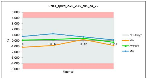
Figure 5-2. Pulse Width Distortion NDD Graph
