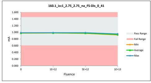
Figure 5-1. Supply Current Disable I<sub>CC1</sub> NDD Graph
