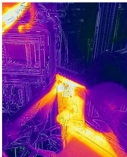
Figure 3-2. INA951-SEP Temperature Reading during SEL Testing
