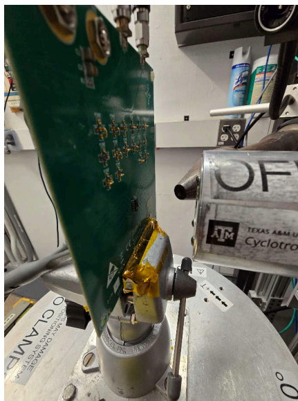
Figure 4-1. THVD9491-SP Evaluation Board in Front of the Heavy-Ion Beam Exit Port at the Texas A&M Cyclotron
