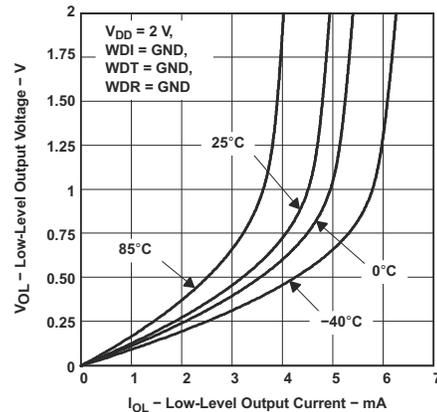
**Figure 6-3. Low-Level Output Voltage vs Low-Level Output Current**
