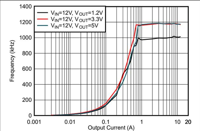
Figure 5-34.  $F_{SW}$  Load Regulation, Mode = DCM,  $F_{SW} = 1200$  kHz
