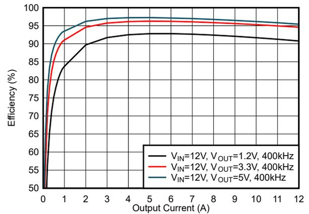
**Figure 5-16. Efficiency, FCCM Mode,  $f_{sw} = 400$  kHz**
