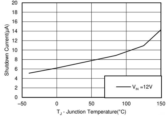
Figure 5-2. Shutdown Current vs Temperature
