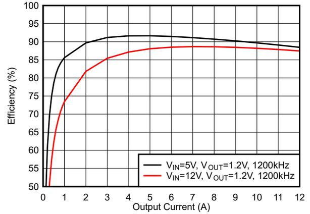
**Figure 5-14. Efficiency, FCCM Mode,  $f_{sw} = 1200$  kHz**
