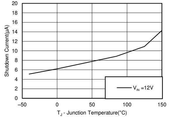
**Figure 5-2. Shutdown Current vs Temperature**
