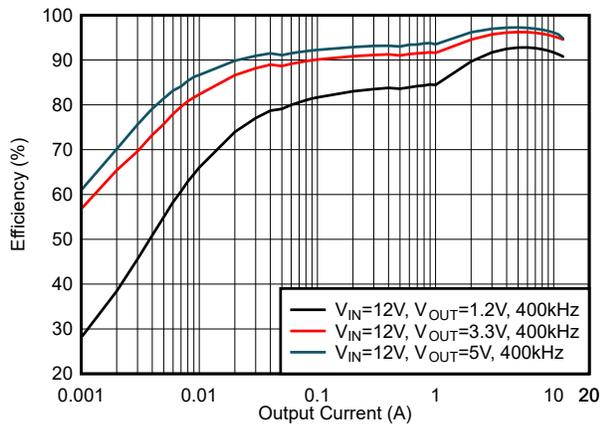
**Figure 5-15. Efficiency, DCM Mode,  $f_{sw} = 400$  kHz**
