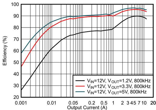
**Figure 5-17. Efficiency, DCM Mode,  $f_{sw} = 800$  kHz**
