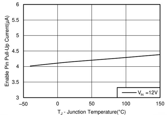
Figure 5-6. Enable Pullup Current, V<sub>EN</sub> = 1.3 V
