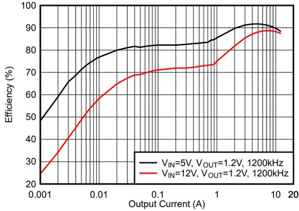
**Figure 5-13. Efficiency, DCM Mode,  $f_{sw} = 1200$  kHz**
