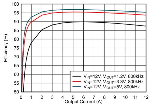
**Figure 5-18. Efficiency, FCCM Mode,  $f_{sw} = 800$  kHz**
