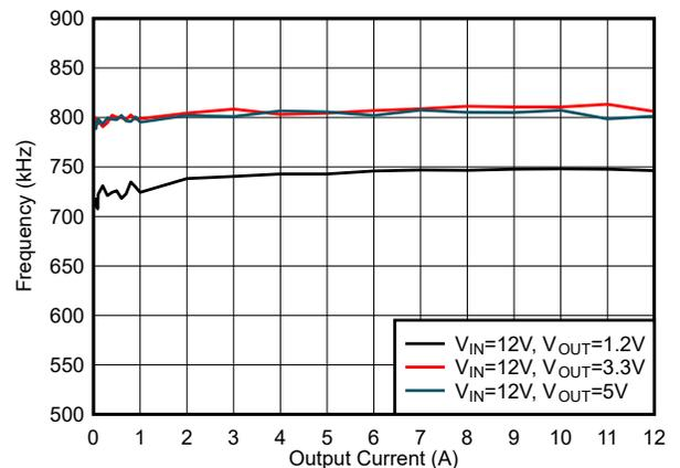
Figure 5-30.  $F_{SW}$  Load Regulation, Mode = FCCM,  $F_{SW} = 800$  kHz
