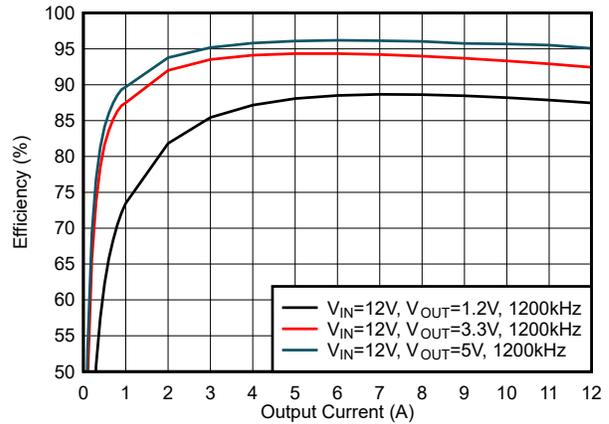
Figure 5-20. Efficiency, FCCM Mode,  $f_{SW} = 1200 \text{ kHz}$
