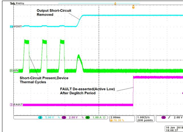
$V_{IN} = 5\text{ V}$ ,  $R_{ILIM} = 20\text{ k}\Omega$
