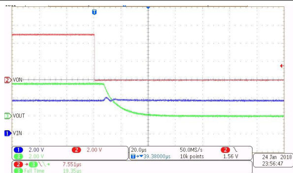
Figure 7-25. Turn-Off at 3.6 V
