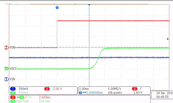
Figure 7-18. Turn-On at 1 V (CT = 1000 pF)
