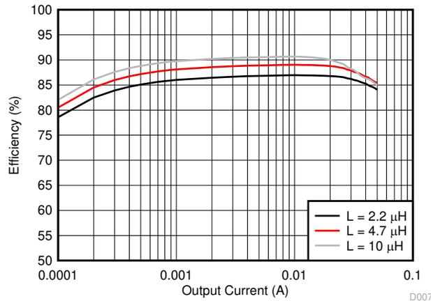
Würth Electronics, 74438335XXX family      2.2  $\mu\text{H}$ , 4.7  $\mu\text{H}$ , 10  $\mu\text{H}$        $V_{IN} = 1.2 \text{ V}$       TPS61322
