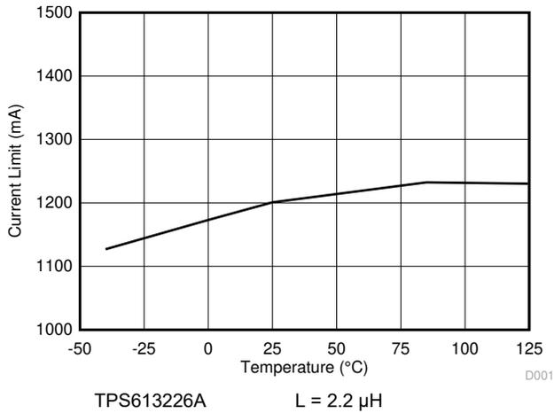
**Figure 6-13. Current Limit with Different Temperature**
