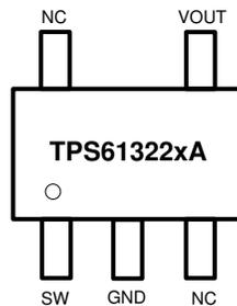
Figure 5-2. DBV Package 5-Pin SOT Top View
