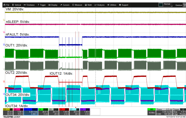
Figure 8-15. Over Current Protection and Recovery
