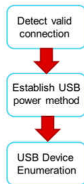
Figure 10-13. Flow of DFP to UFP Configuration
