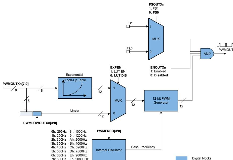
**Figure 6-6. Output Current Control Path in FAIL-SAFE State**
