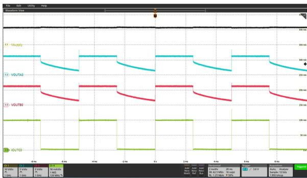
Ch1 =  $V_{(SUPPLY)}$     Ch2 =  $V_{(OUTA0)}$     Ch3 =  $V_{(OUTB0)}$
