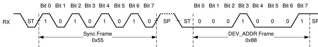
Figure 6-13. Synchronization Byte
