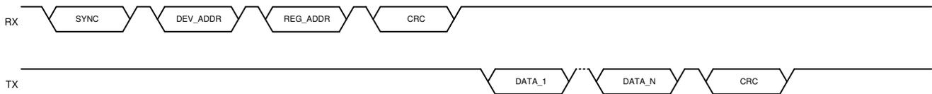
**Figure 6-17. Multiple Data Bytes Read in Burst Mode**
