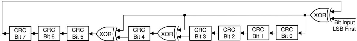
Figure 6-7. CRC Algorithm Diagram
