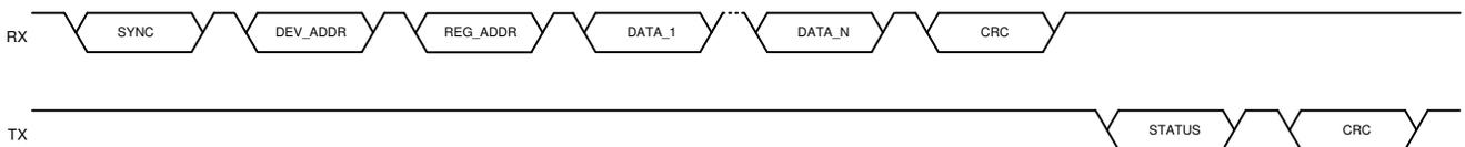
Figure 6-16. Multiple Data Bytes Write in Burst Mode
