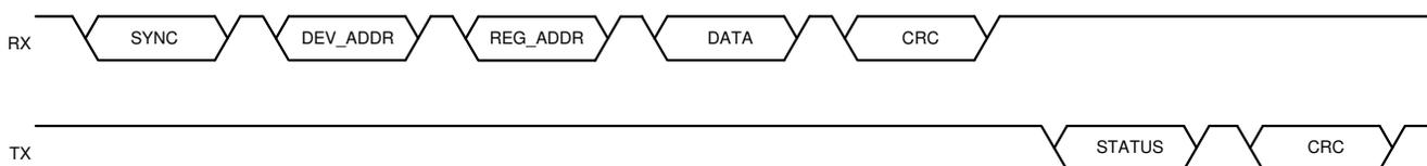
**Figure 6-11. Single-Byte Write Command with Status Feedback**
