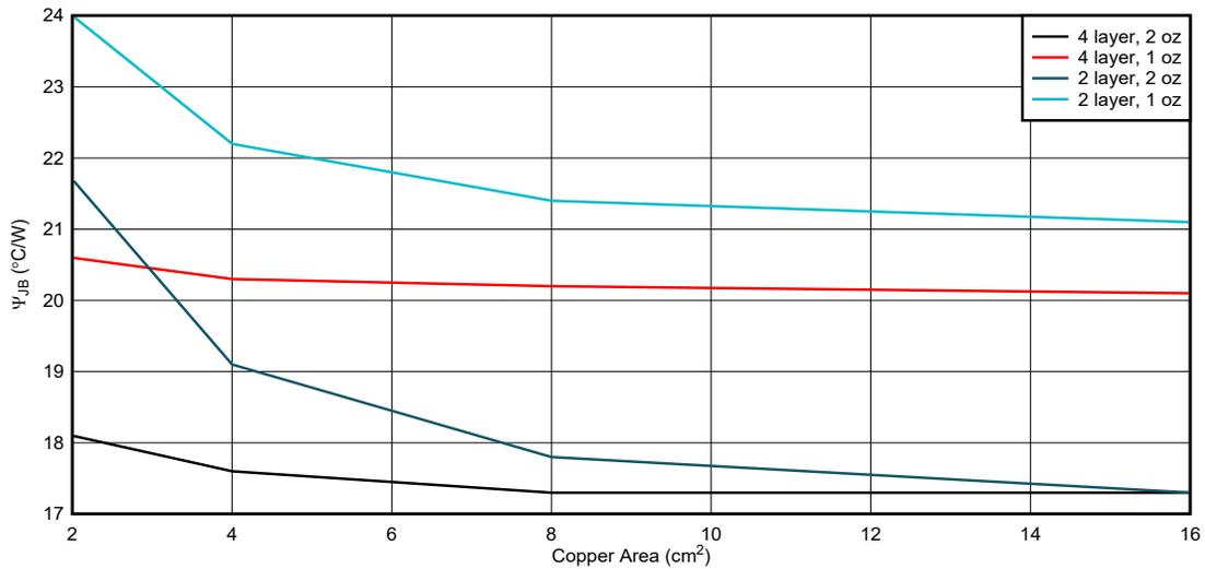
**Figure 9-13. WSON, junction-to-board characterization parameter vs copper area**
