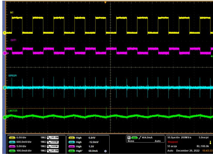
**Figure 9-6. PWM Operation at VM = 1.65 V**
