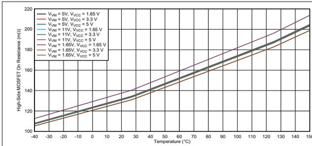
Figure 7-6. High-Side MOSFET ON Resistance (RTE Package)
