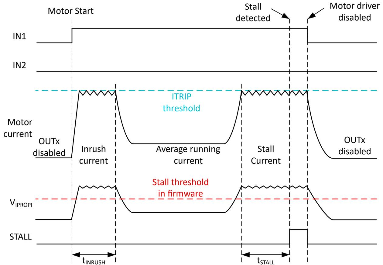
**Figure 9-5. Motor Current Profile with STALL Signal**
