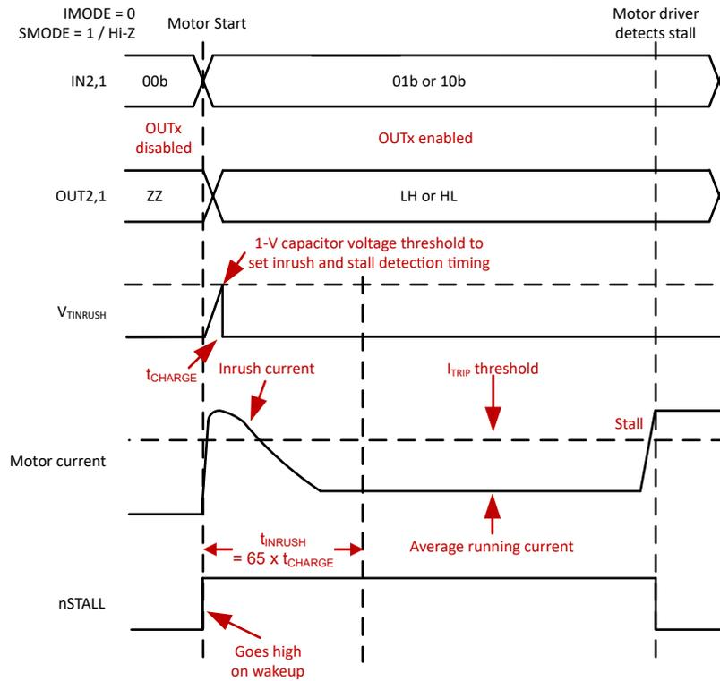
**Figure 8-8. Stall Detection with nSTALL indication only**
