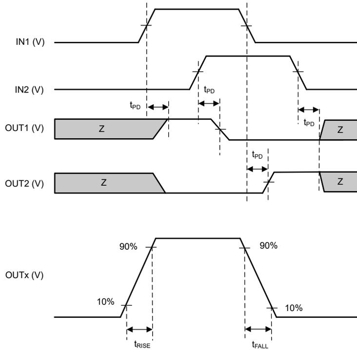
**Figure 7-1. Input-to-Output Timing**
