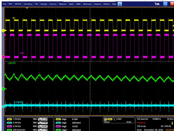
Figure 9-8. PWM Operation at  $V_M = 11\text{ V}$
