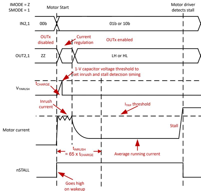
**Figure 8-9. Stall regulation with current regulation during inrush**
