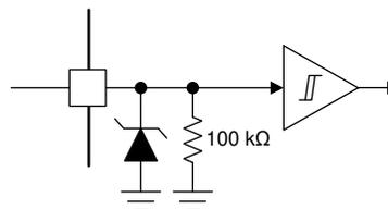
**Figure 8-14. Logic-level input**
