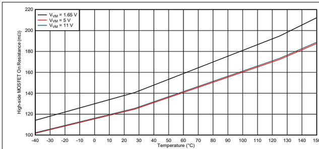
**Figure 7-2. High-Side MOSFET ON Resistance (DSG Package)**
