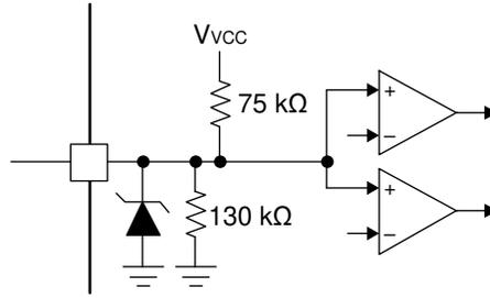
**Figure 8-15. Tri-level input**
