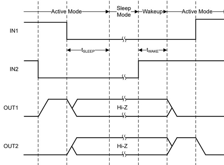
**Figure 8-13. Sleep Mode Entry and Wakeup Timing Diagram**
