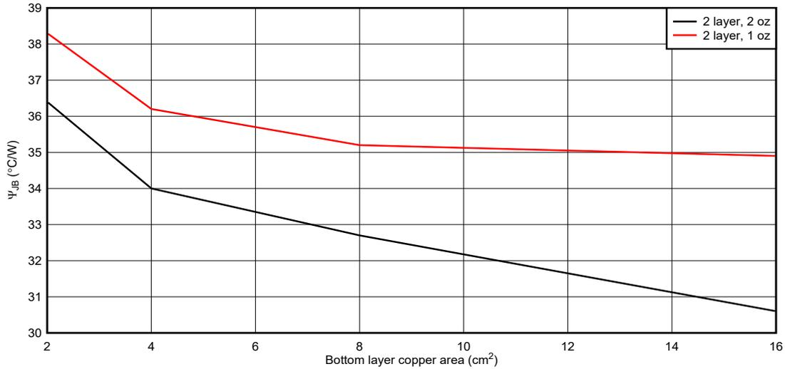
**Figure 9-15. WQFN, junction-to-board characterization parameter vs copper area**
