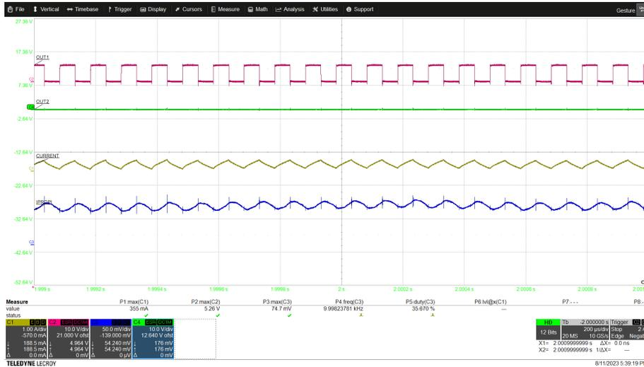
**Figure 9-7. PWM Operation at VM = 5 V**
