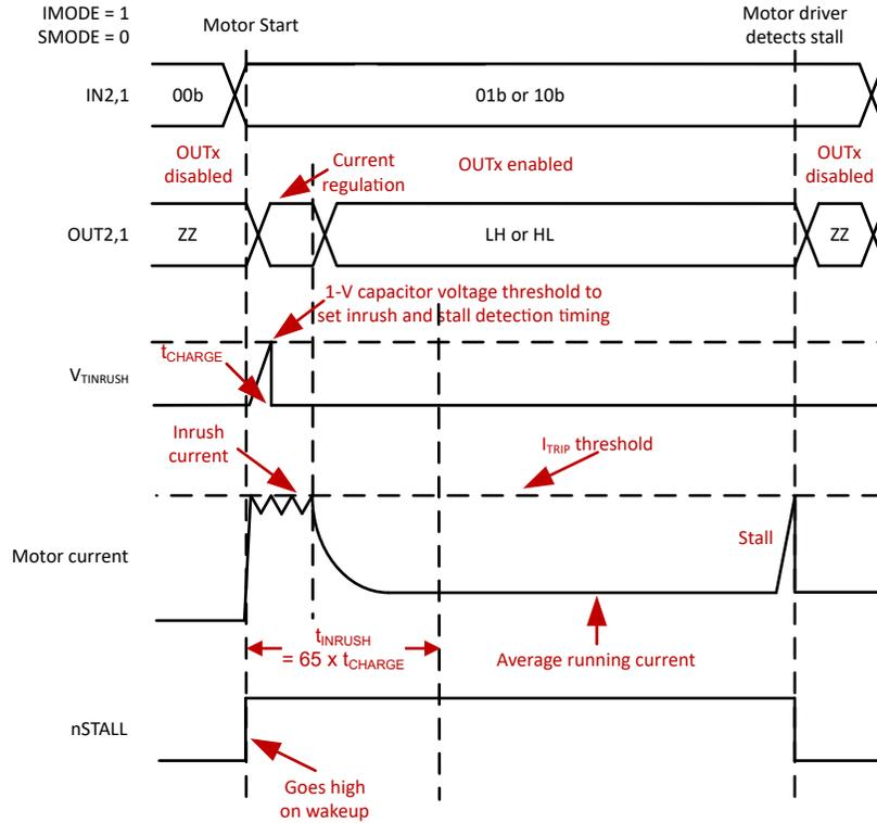
Figure 9-4. Example timing diagram for hardware stall detection
