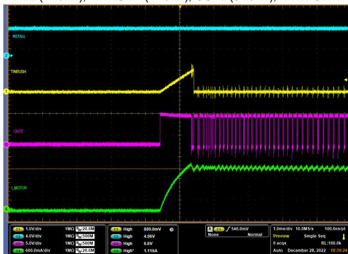
Figure 9-9. Stall Detection with  $IMODE = \text{Hi-Z}$ ,  $SMODE = 1$
