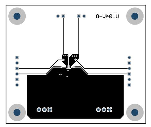
Figure 3. Bottom Layer Routing
