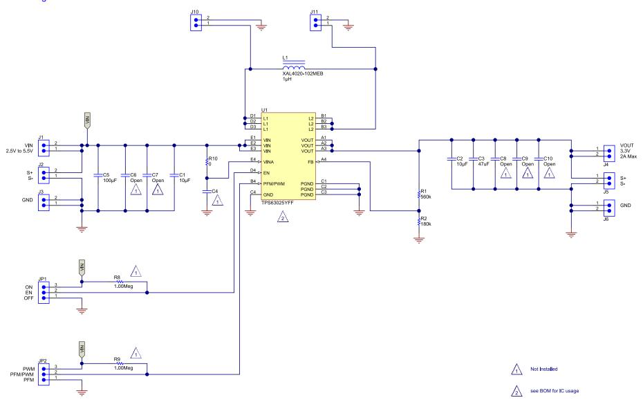
Figure 4. TPS63025xEVM-553 Schematic
