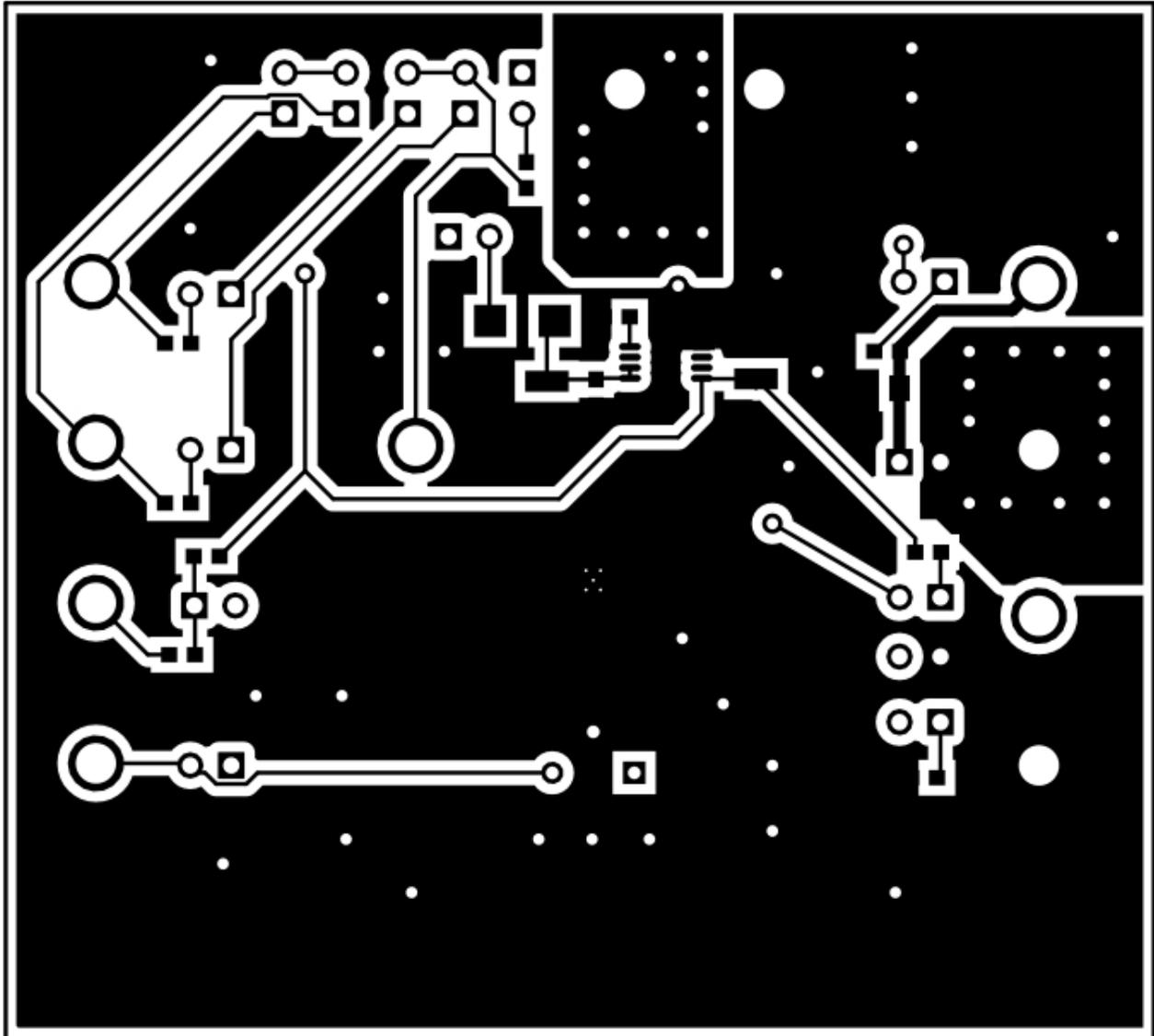
Figure 5. TPS1H200-Q1 EVM Bottom Layer (Bottom View)
