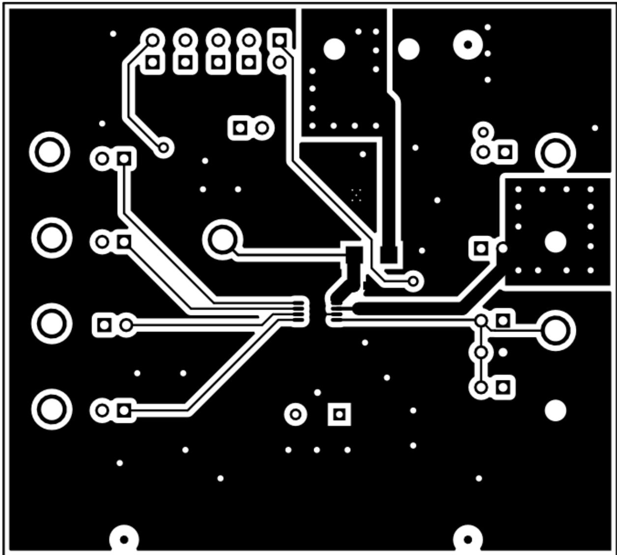
Figure 4. TPS1H200-Q1 EVM Top Layer (Top View)
