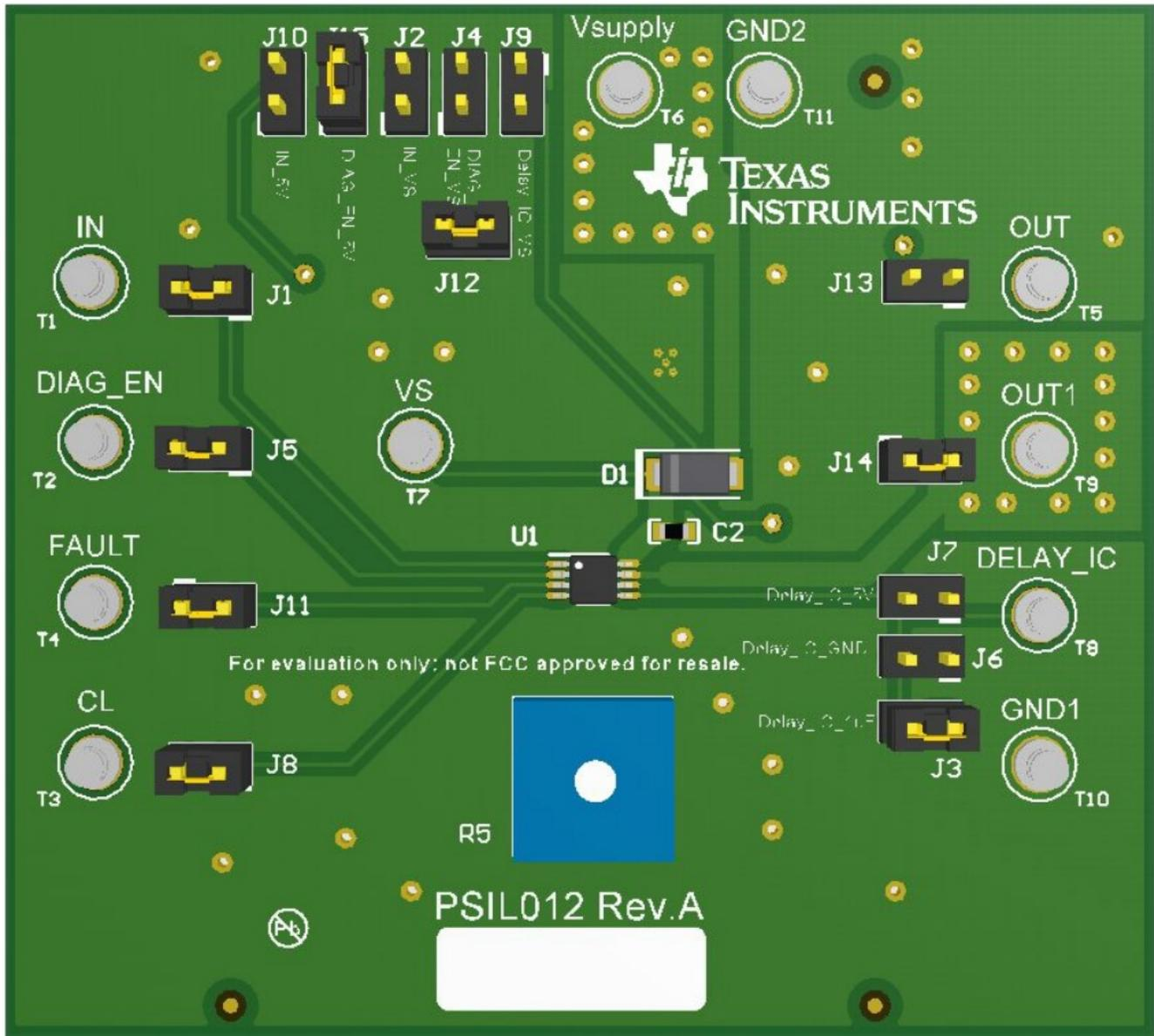
Figure 3. TTPS1H200-Q1 EVM Component Placement (Top View)
