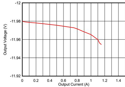
Figure 4-22. Load Regulation ( $V_{OUT} = -12\text{ V}$ )
