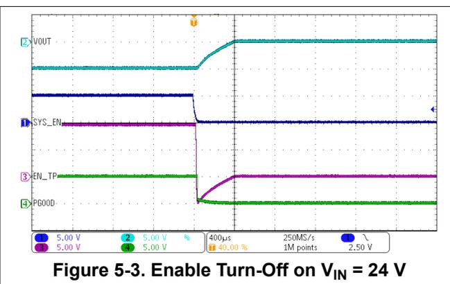
Figure 5-3. Enable Turn-Off on  $V_{IN} = 24\text{ V}$
