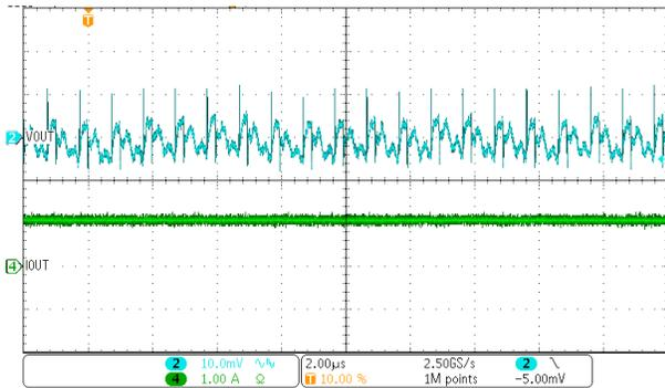
Figure 4-17. Output Ripple Waveform
