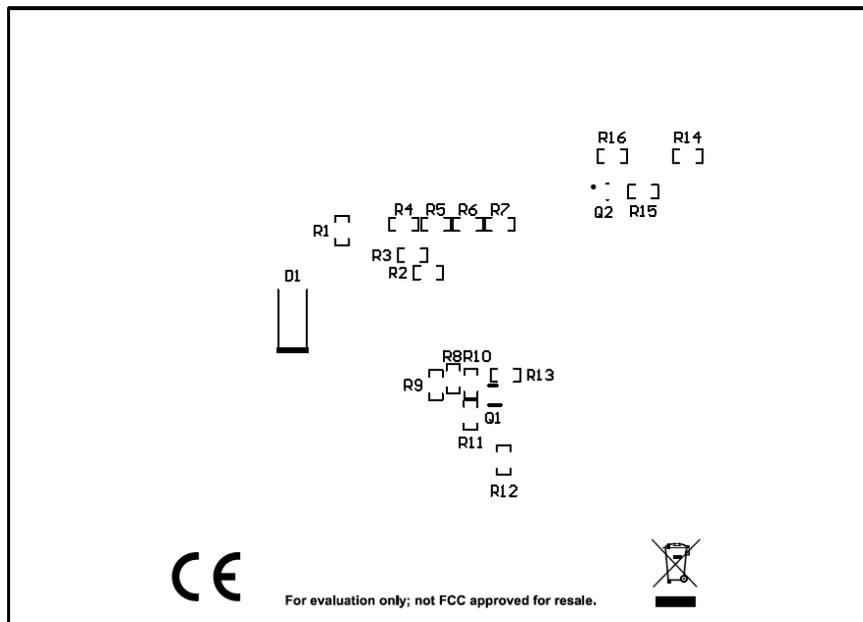
Figure 6-6. Bottom Layer Silk Screen (Bottom View)
