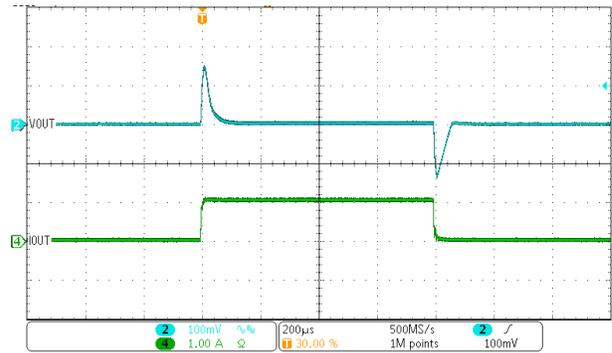
Figure 4-12. Transient Response Waveform
