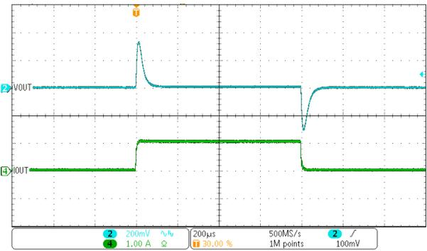
Figure 4-24. Transient Response Waveform
