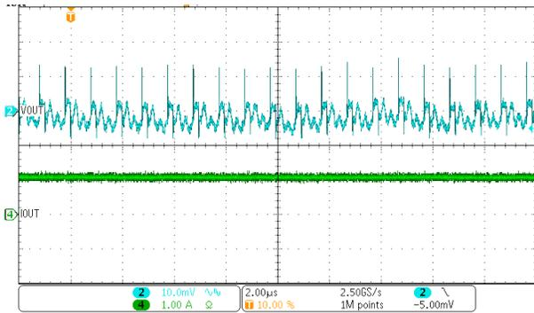
Figure 4-23. Output Ripple Waveform
