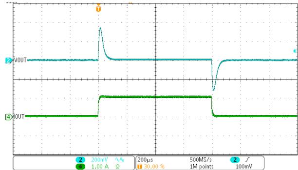
Figure 4-18. Transient Response Waveform
