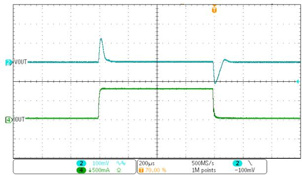
Figure 4-6. Transient Response Waveform
