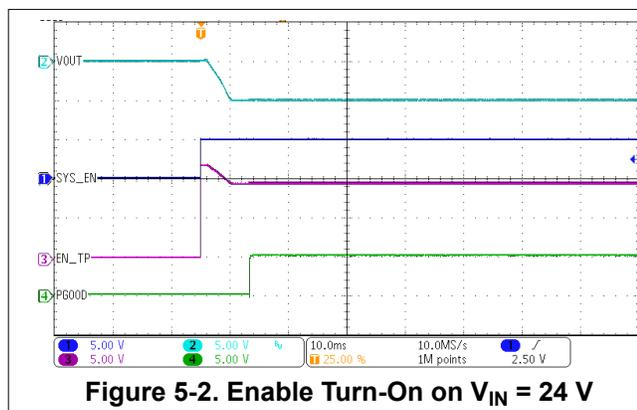
Figure 5-2. Enable Turn-On on  $V_{IN} = 24\text{ V}$
