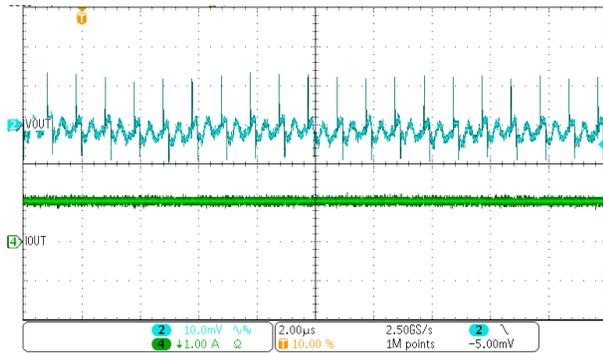
Figure 4-11. Output Ripple Waveform
