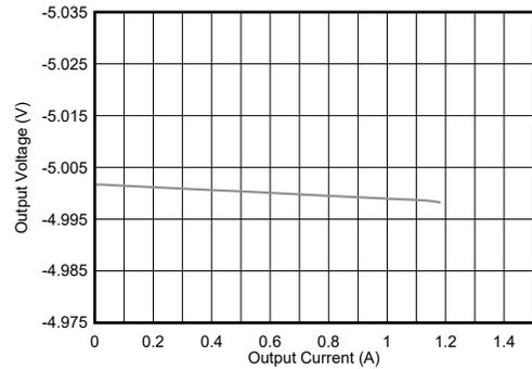
Figure 4-10. Load Regulation ( $V_{OUT} = -5\text{ V}$ )
