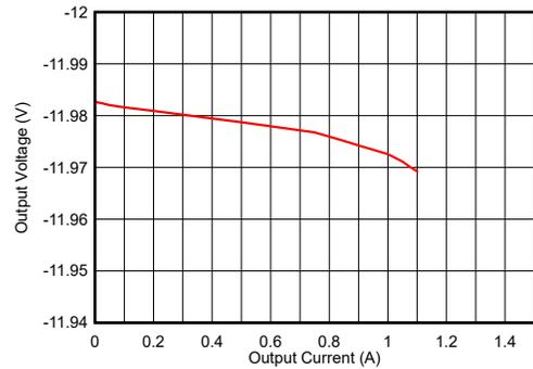
Figure 4-16. Load Regulation ( $V_{OUT} = -12\text{ V}$ )
