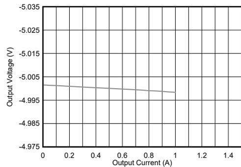
Figure 4-4. Load Regulation ( $V_{OUT} = -5\text{ V}$ )
