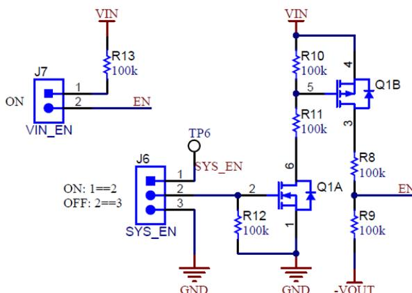
Figure 5-1. Enable Level-Shifter
