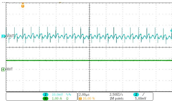
Figure 4-5. Output Ripple Waveform
