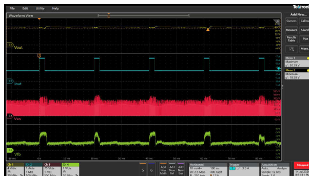
Figure 3-61. VIN=90Vac (2x Rated Current for 2ms, 0.9x Rated Current for 18ms)
