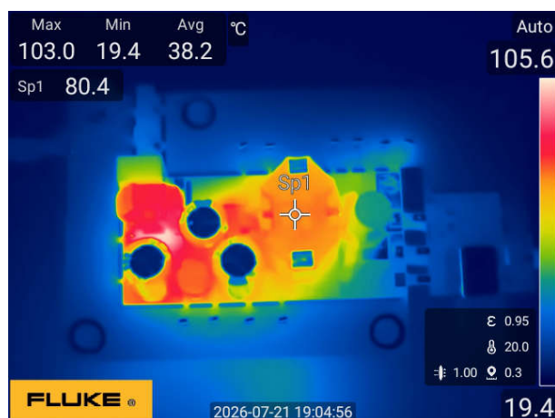
Figure 3-78. Top Side at 90Vac-to-20V/3.25A
