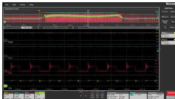
Figure 3-63. VIN=90Vac (2x Rated Current for 2ms, 0.9x Rated Current for 18ms) - Zoomed
