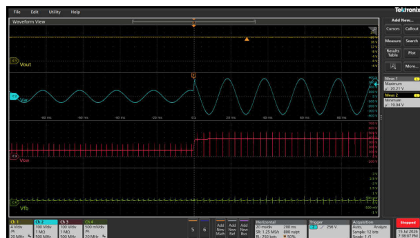
Figure 3-58. Line Transient from 90Vac to 264Vac at 20V/No Load
