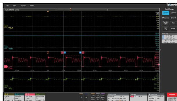
Figure 3-38. 230Vac/40W (87kHz 6 th Valley Switching/ Vfb - 1.73V)
