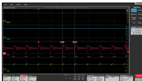
Figure 3-37. 230Vac/16W (52kHz Frequency-Foldback/ Vfb - 1.46V)
