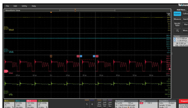
Figure 3-39. 230Vac/65W (106kHz 3 rd Valley Switching/Vfb - 1.93V)
