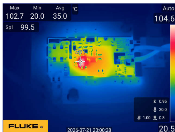
Figure 3-85. Bottom Side at 264Vac-to-20V/3.25A
