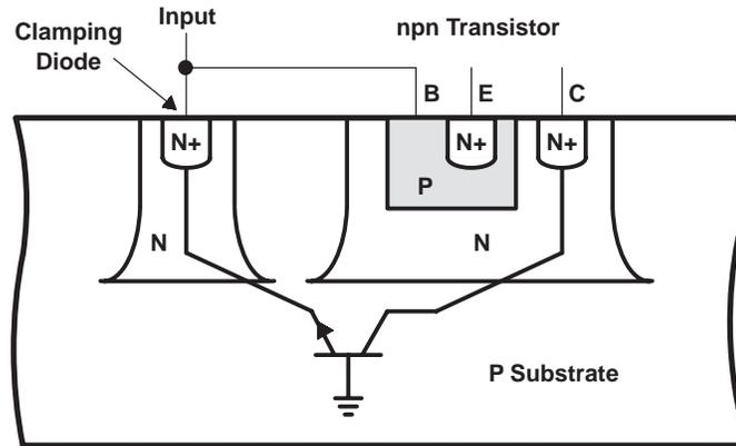
**Figure 15. Parasitic Transistors in Bipolar Circuits**
