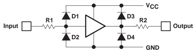
**Figure 13. Protection Circuits for Integrated Circuits**
