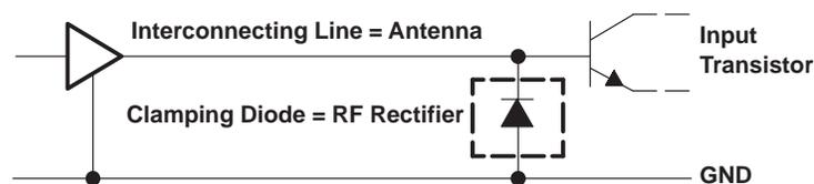
**Figure 20. Rectification of High-Frequency Interference Signals**
