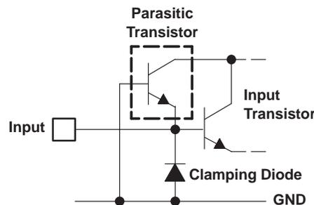
**Figure 16. Input Circuit With Parasitic Transistor**
