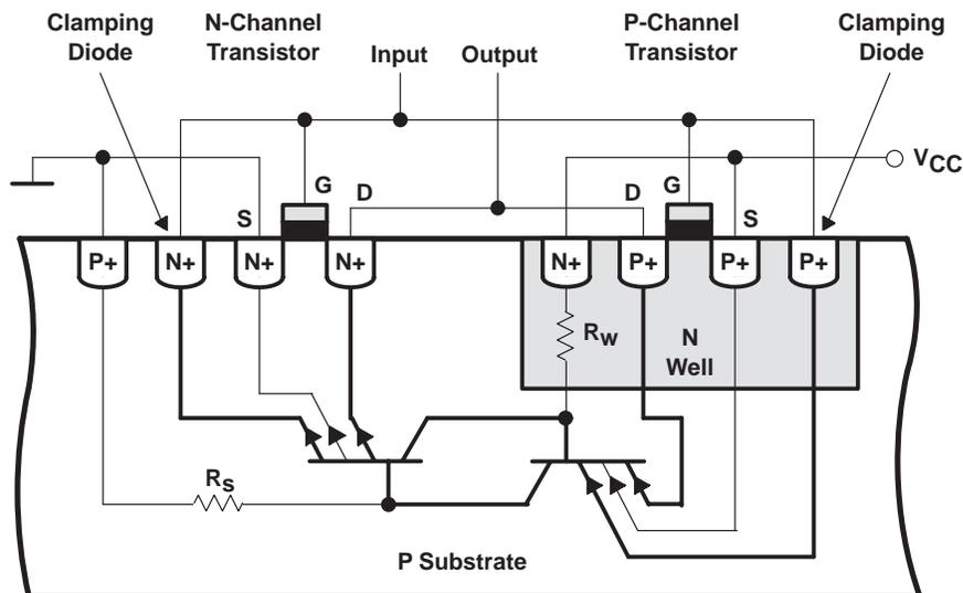
Figure 1. Parasitic Transistors in a CMOS Circuit
