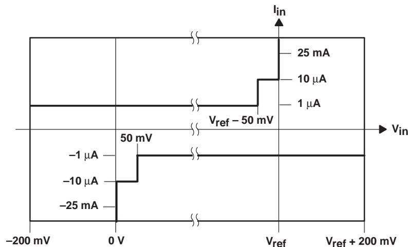
Figure 18. Characteristics of Voltage Limiter TL7726
