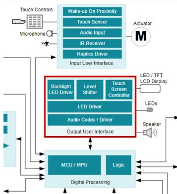
TI Applications diagram – Vacuum robot
