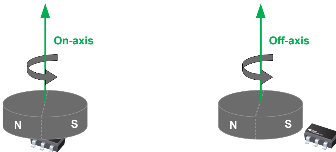
Figure 7-9. On-Axis vs Off-Axis Angle Measurements
