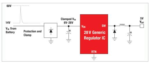
*Figure 3a*. A generic 24V regulator with in a battery-supplied system with voltage clamp for protection against input voltage surges.
