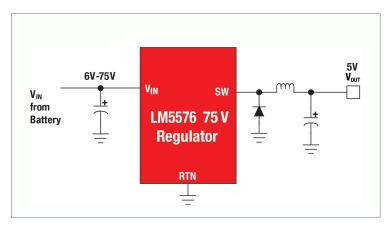
Figure 3b. Regulator with high-voltage rating eliminates the need for input clamp circuit.
