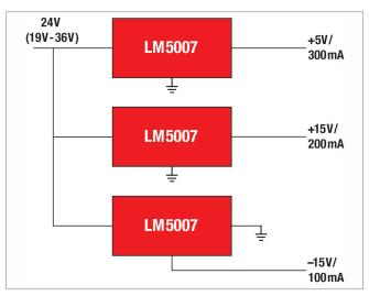
*Figure 8*. A block diagram for 24V to 5V/15V/–15V power conversion using a high-voltage regulator IC. High-voltage rating allows for input voltage variation and design margin.
