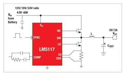
*Figure 3c*. A buck converter for a USB charging port can operate from 12V/24V automotive rails or 19V laptop charging rails.
