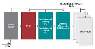
Figure 1: Standard 24V PLC system.
