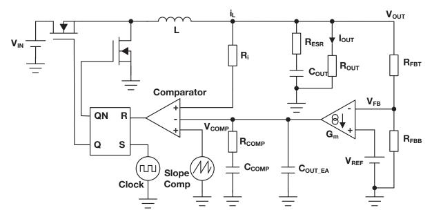
Figure 7. Block diagram of a typical PCM buck converter.
