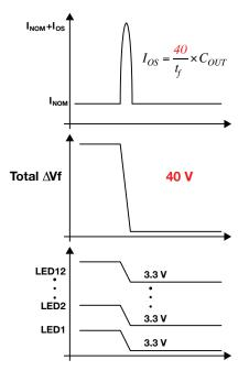
Figure 3. Overshoot current with all 12 LEDs on the LMM turning off.
