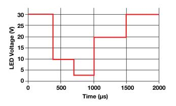
Figure 2. Variation of LED voltage (dynamic LED load).
