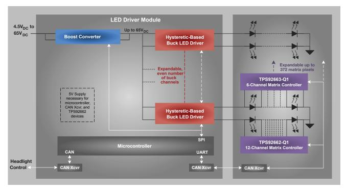
Figure 10. Suggested ECU architecture with an LMM.
