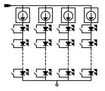
Figure 1. Simplified block diagram of an LMM.
