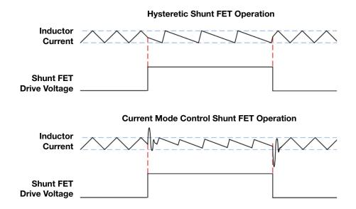
Figure 9. Difference between HC and PCM DC/DC LED drivers with shunt FET dimming.
