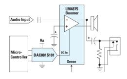
Figure 2. DC-Control of an Audio Amplifier
