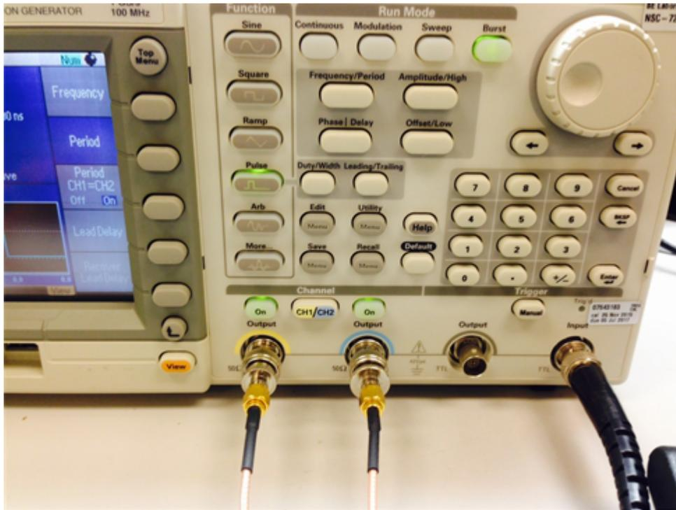
Figure 7. Tektronix AFG3102 Connections
