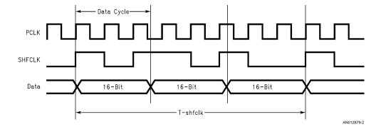
FIGURE 2. 640x480 STN-DD Panel PCLK vs. SHFCLK
