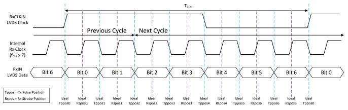
Figure 4. Internal PLL Determines Strobe Positions for the Serialized LVDS Bits
