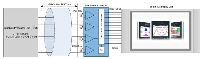
Figure 3. Channel Link I Rx Device Used as a Serial-to-Parallel Bridge
