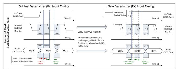
Figure 9. Improving RSKM with Small Left Margin at Receiver Input
