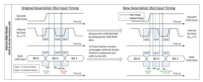
Figure 10. Improving RSKM with Small Right Margin at Receiver Input
