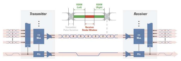
Figure 5. Receiver Skew Margin Illustration
