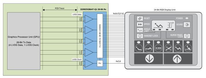
Figure 8. GPU Connection Diagram to DS90CR286AT-Q1 Receiver
