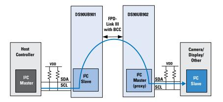
Figure 5. Accessing a Remote I<sup>2</sup>C Slave Using the FPD-Link III Bidirectional Control Channel
