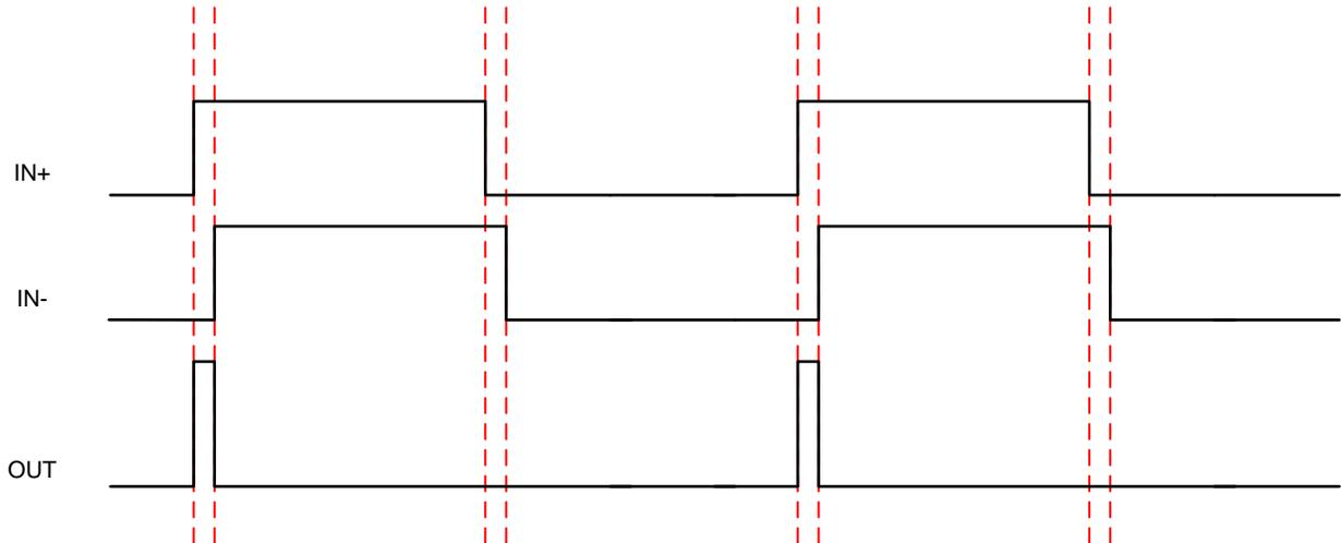
Figure 10. Timing Diagram To Create Short Pulses
