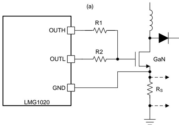
**Figure 7. Source Resistor Current Sense A Configuration**
