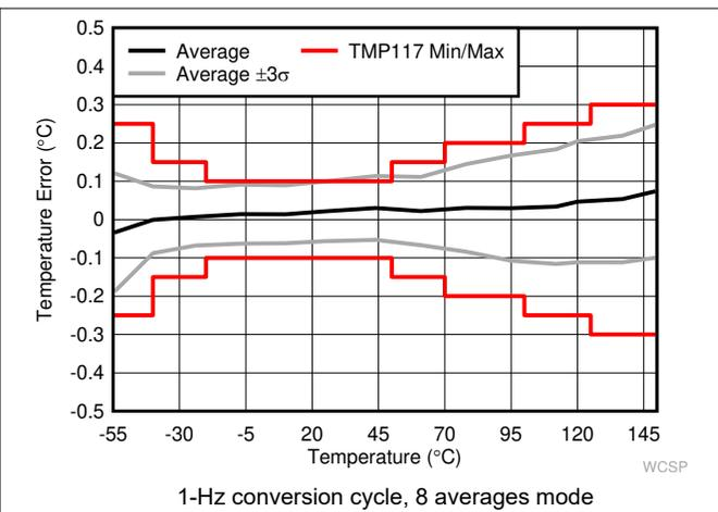
Figure 6-3. YBG Package Temperature Error vs Temperature
