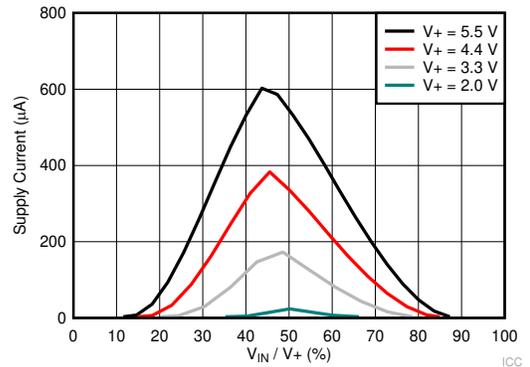
Figure 6-13. Supply Current vs Input Cell Voltage
