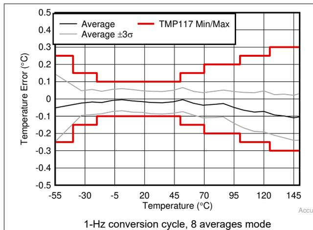
Figure 6-2. DRV Package Temperature Error vs Temperature
