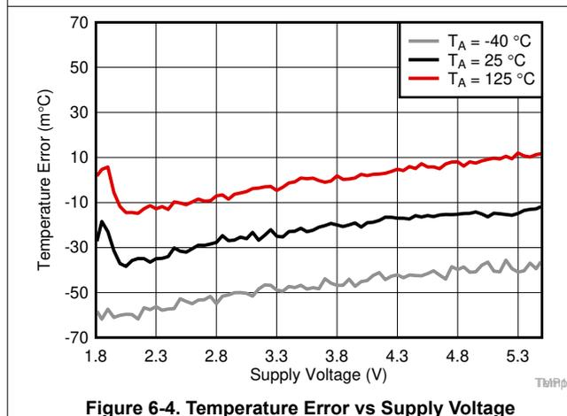
Figure 6-4. Temperature Error vs Supply Voltage
