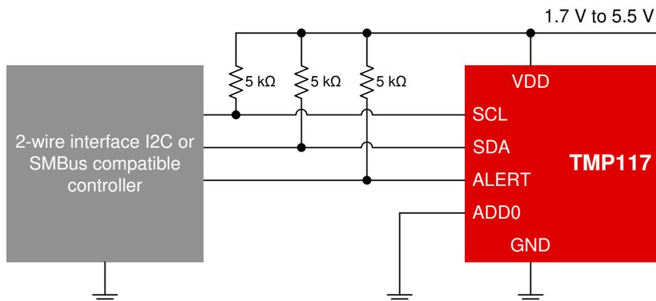
Figure 8-1. Typical Connections
