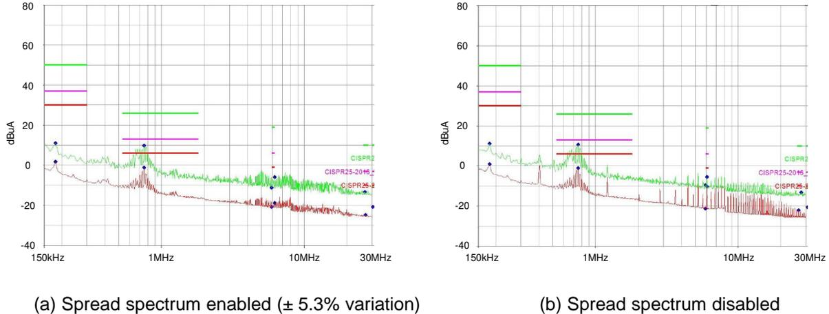
**Figure 8. Conducted Emissions: Spread Spectrum**
