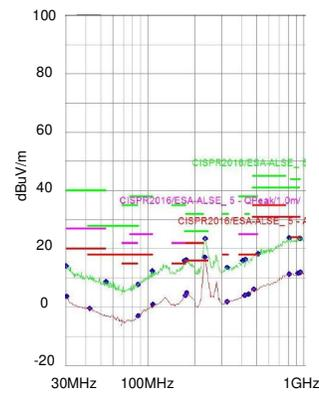
(b) C8 and C9 on footprint of C10 and C11
