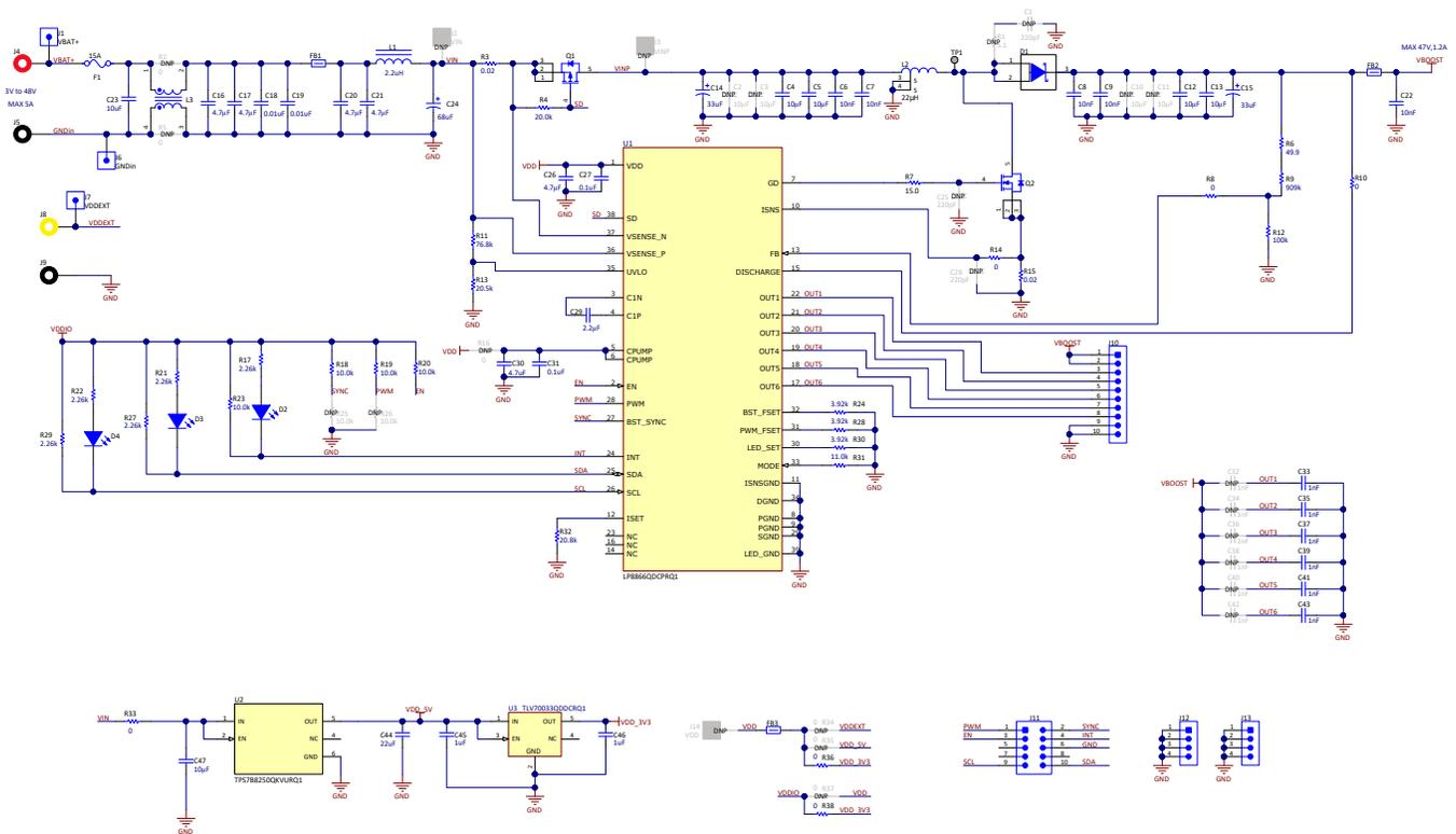
Figure 1. LP8866-Q1 Reference Design Schematic
