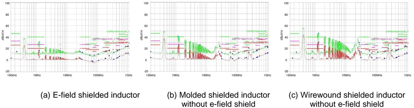
**Figure 16. Radiated Emissions: Inductor Selection**
