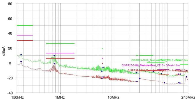
(a) With 1-nF capacitors from current sinks to ground
