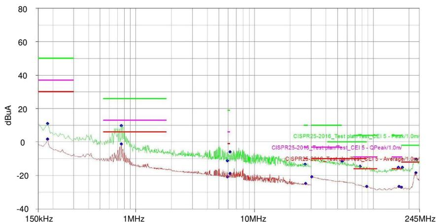
Figure 4. CISPR 25 Class 5 Conducted Emission Limits And Measurement Results
