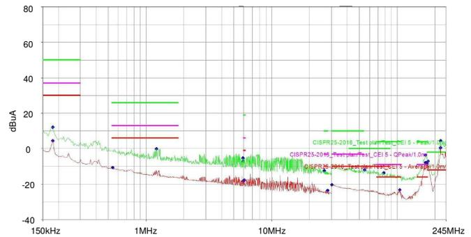
(b) Without 1-nF capacitors from current sinks to ground
