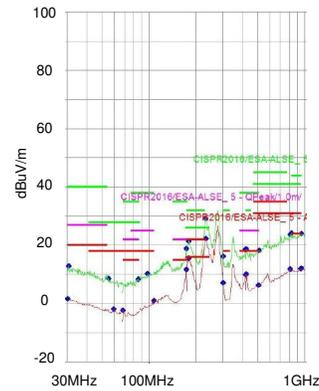
(b) Without 1-nF capacitors from current sinks to ground
