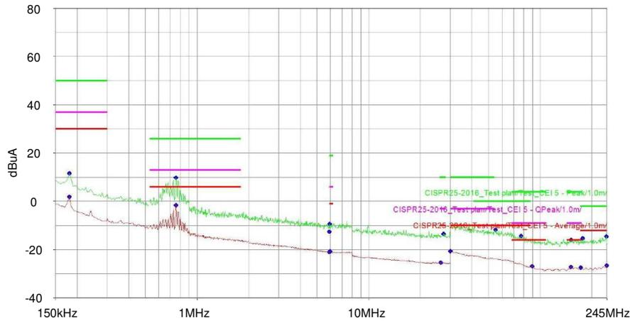
**Figure 5. CISPR 25 Class 5 Conducted Emission Limits And Ambient Noise**
