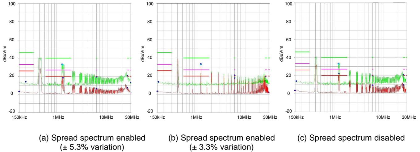
**Figure 7. Radiated Emissions: Spread Spectrum**
