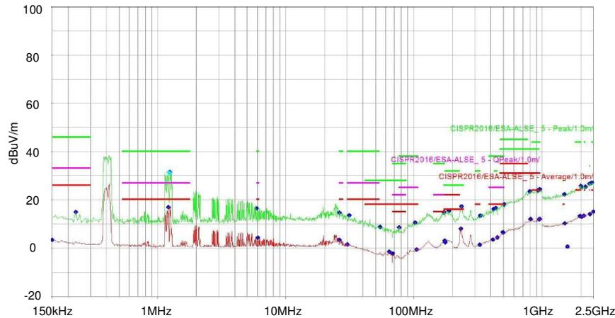
**Figure 6. CISPR 25 Class 5 Radiated Emission Limits And Measurement Results**
