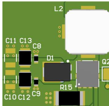
Figure 13. Boost Critical Loop Layout
