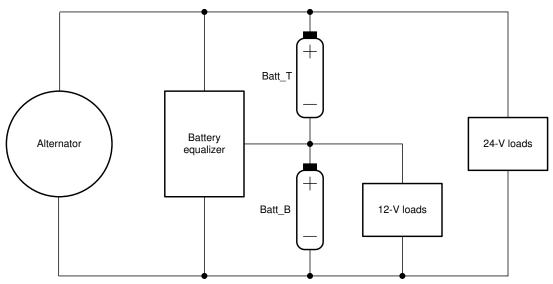
Figure 1-1. Power System of Commercial Vehicles
