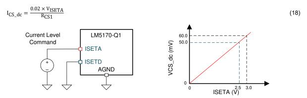
Figure 2-6. ISETA vs VCS\_dc Graph of LM5170-Q1
