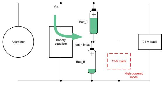
Figure 1-3. Constant Current Mode of Battery Equalizer
