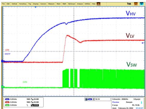
Figure 3-5. Start-up Sequence of Buck Converter
