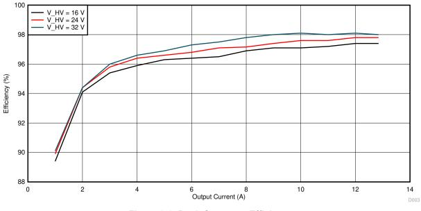
Figure 3-2. Buck Converter Efficiency
