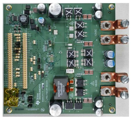
Figure 3-1. Test Board (Texas Instruments LM5170EVM-BIDIR Modified)
