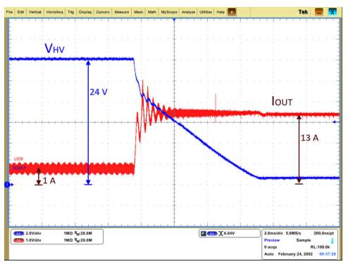
Figure 3-4. Input Voltage and Output Current Waveform in Constant Current Mode
