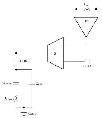
Figure 2-2. Inner Current Loop Control in LM5170-Q1
