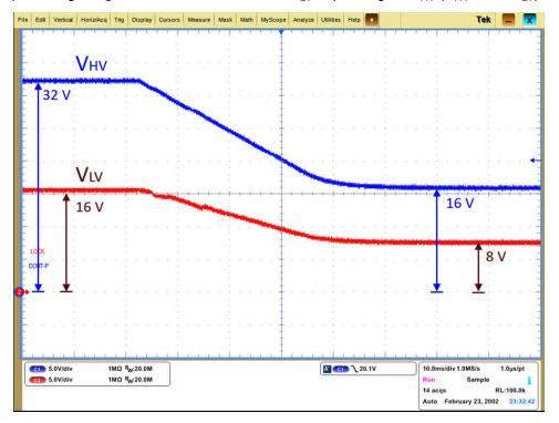
During constant voltage mode of battery equalizer, buck converter should keep constant ratio between input voltage and output voltage. Figure 3-3 shows transition of  $V_{LV}$  depending on  $V_{HV}$  ( $V_{HV}$  = 2 ×  $V_{LV}$ ).
