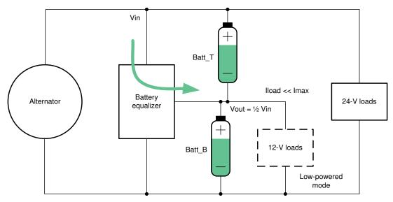
Figure 1-2. Constant Voltage Mode of Battery Equalizer
