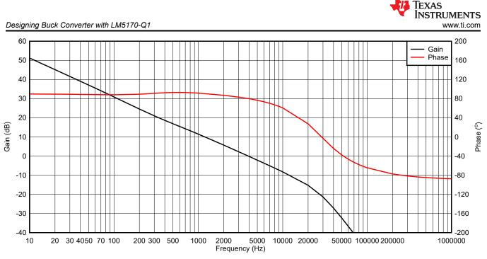
Figure 2-5. Bode Plot of Outer Voltage Loop
