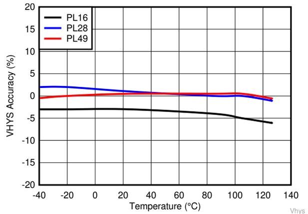
**Figure 6-11. Input Threshold  $V_{IT}$ . Hysteresis Accuracy for TPS3840PLXX**
