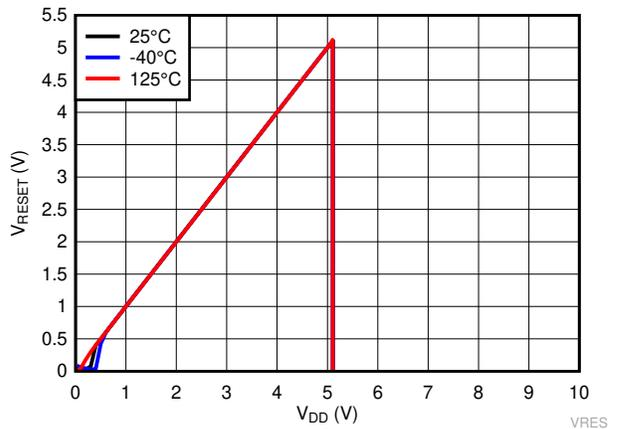
**Figure 6-15. Output Voltage vs Input Voltage for TPS3840PH49**
