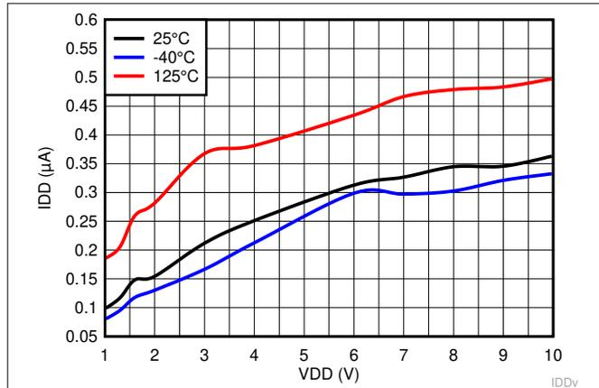
**Figure 6-4. Supply Current vs Supply Voltage for TPS3840DL49**
