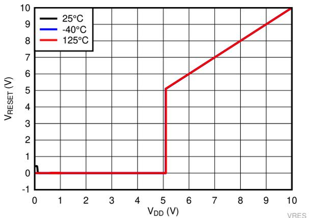
**Figure 6-14. Output Voltage vs Input Voltage for TPS3840PL49**
