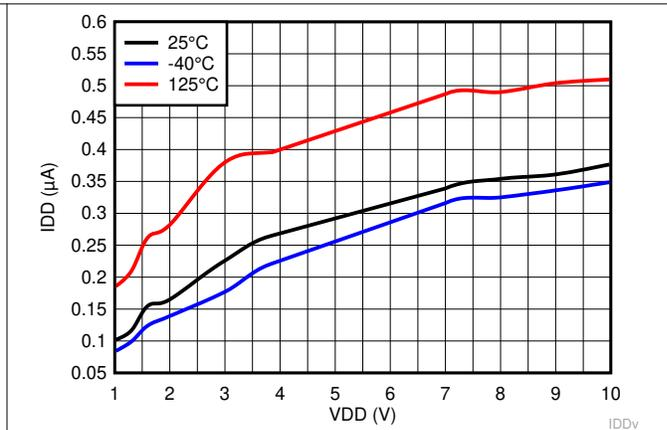
**Figure 6-5. Supply Current vs Supply Voltage for TPS3840PL49**
