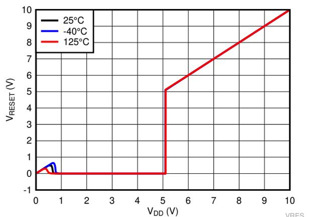
**Figure 6-13. Output Voltage vs Input Voltage for TPS3840DL49**
