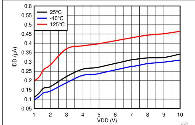
**Figure 6-6. Supply Current vs Supply Voltage for TPS3840PH49**
