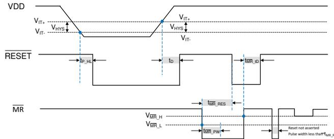
Figure 7-3. Timing Diagram  $\overline{MR}$  and  $\overline{RESET}$  (TPS3840DL)
