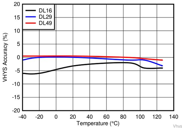
**Figure 6-10. Input Threshold  $V_{IT}$ . Hysteresis Accuracy for TPS3840DLXX**
