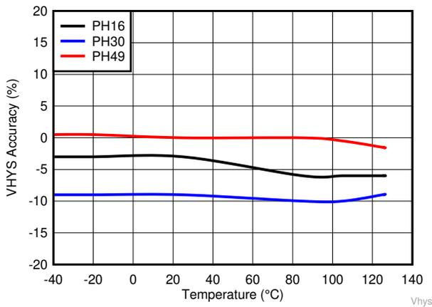
**Figure 6-12. Input Threshold  $V_{IT}$ . Hysteresis Accuracy for TPS3840PHXX**
