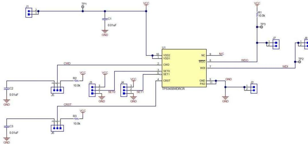
Figure 2. TPS3430EVM Schematic
