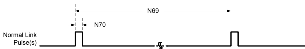
Figure 27-38. 10Base-TX Normal Link Pulse Timing
