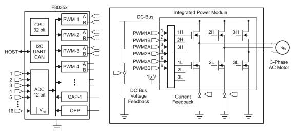
A Note that the dcbus return current is obtained through the summation of three phase currents in R1.1.
