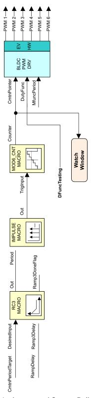
Figure 13. Level 1 - Incremental System Build Block Diagram
