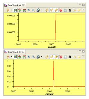
Figure 16. (a) mod6 Counter (b) Impulse Output, dlog.prescalar = 3
