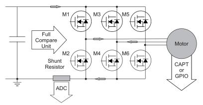
Figure 5. Three Phase Inverter
