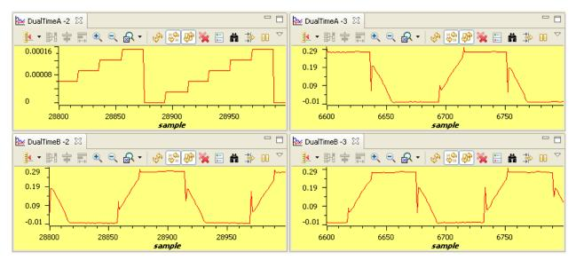
Figure 24. (a) mod6 Counter, (b)BemfA, (c) BemfB (c)BemfC (under no-load at 0.5pu speed, Vdcbus = 160 V)
