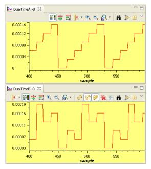
Figure 19. (a) mod6 Counter, (b) HallGpioAccepted (dlog.prescalar = 25 and Vdcbus = 160 V)
