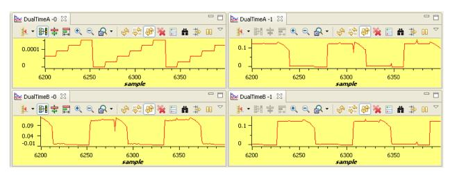
Figure 17. (a) mod6 Counter, (b) BemfA, (c) BemfB and (d)BemfC ( dlog.prescalar = 25 and Vdcbus = 160 V)
