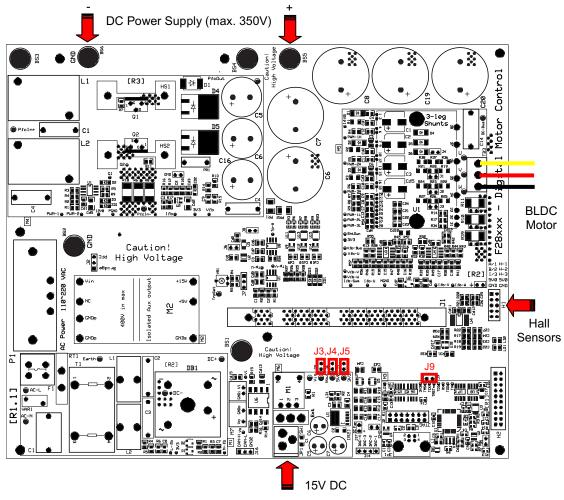
Figure 11. Using External DC Power Supply to Generate DC-Bus for the Inverter
