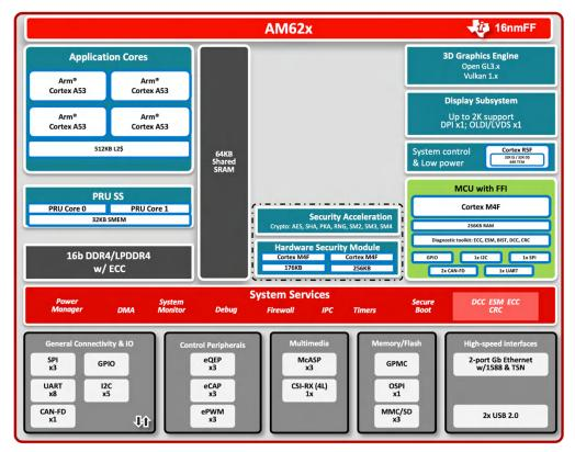
Figure 1-1. Block Diagram of the Sitara<sup>™</sup> AM62x Processors
