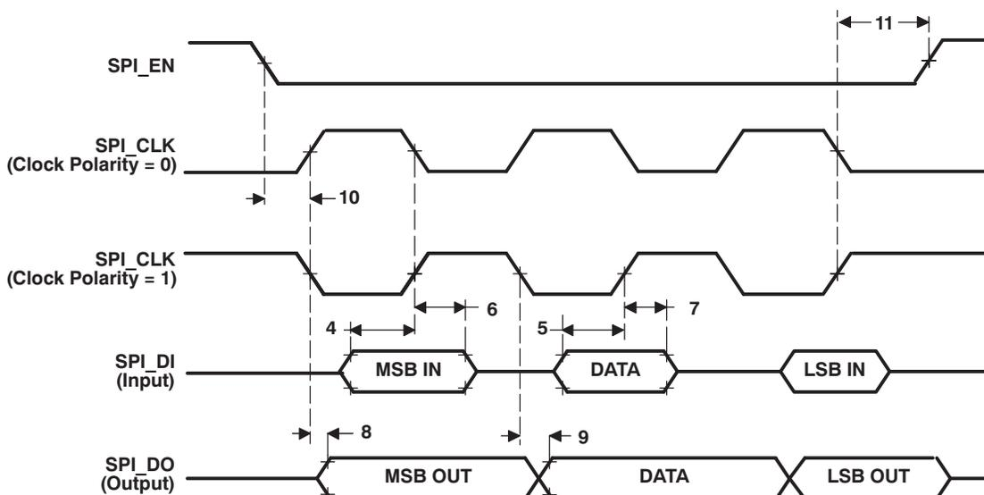
**Figure 5-37. SPI Master Mode External Timing (Clock Phase = 0)**
