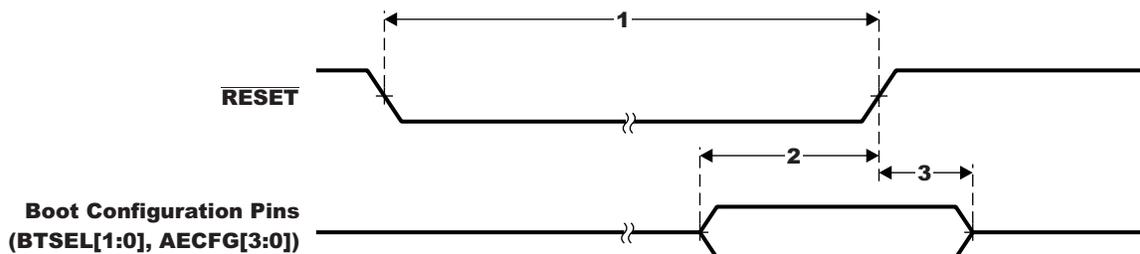
Figure 5-4. Reset Timing
