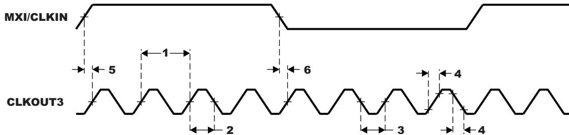
**Figure 5-11. CLKOUT3 Timing**
