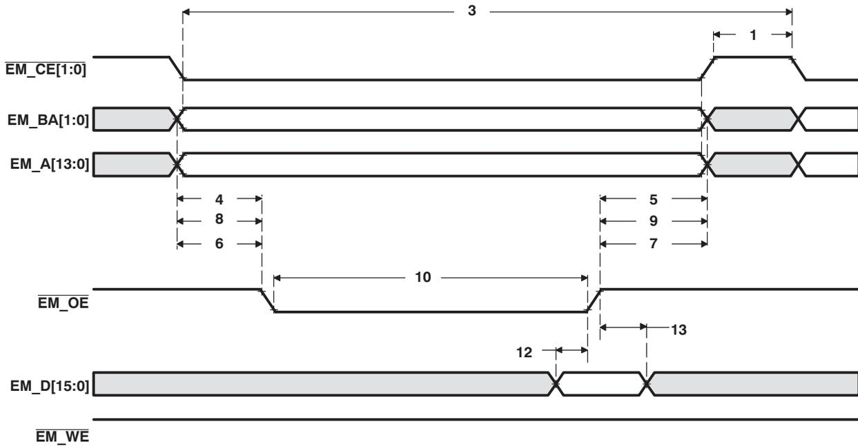
**Figure 5-14. Asynchronous Memory Read Timing for EMIF**
