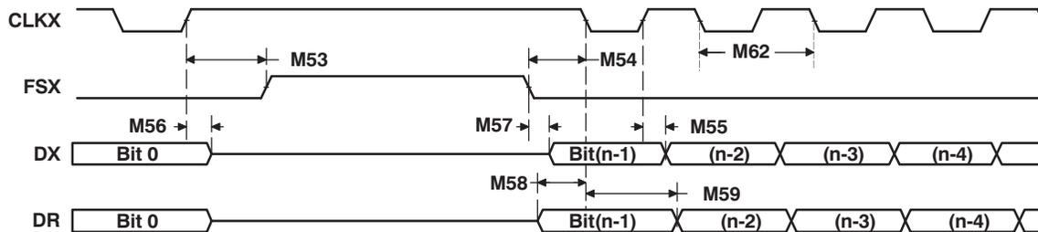
**Figure 5-45. ASP as SPI: CLKSTP = 11b, CLKXP = 1**
