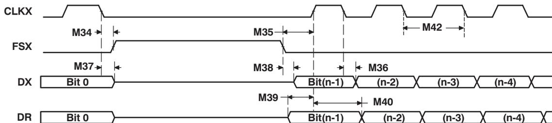
**Figure 5-43. ASP as SPI: CLKSTP = 11b, CLKXP = 0**
