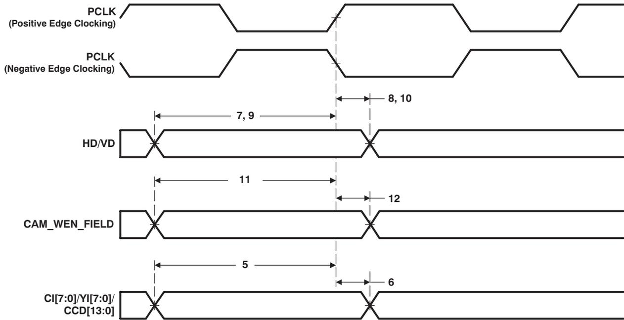
Figure 5-24. VPFE (CCD) Slave Mode Input Data Timing
