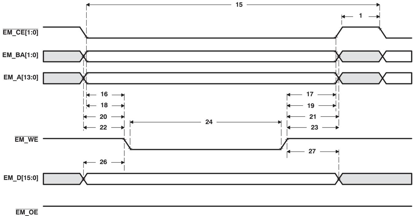
Figure 5-15. Asynchronous Memory Write Timing for EMIF
