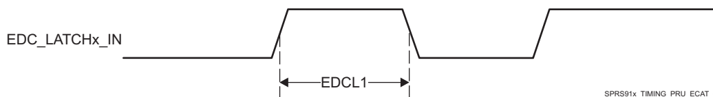
Figure 5-120. PRU-ICSS ECAT LATCHx_IN Timing
