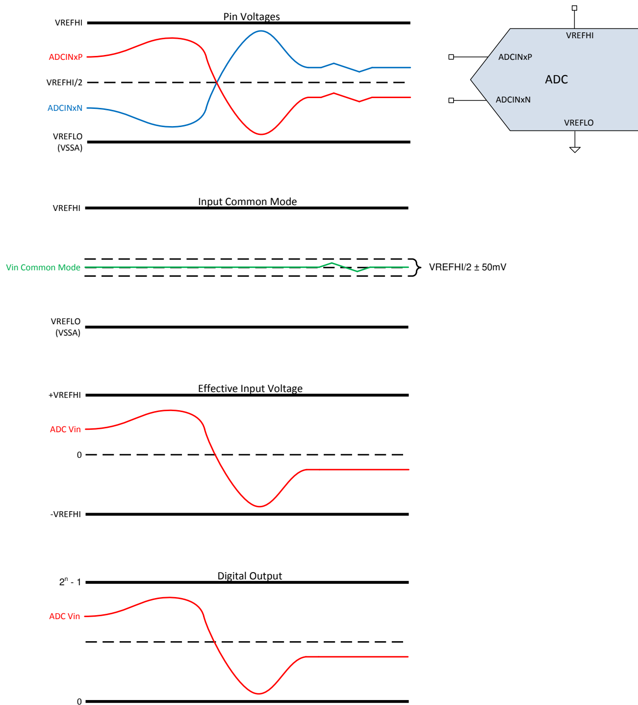
Figure 6-36. Differential Signaling Mode
