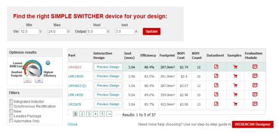
Figure 1. Enter Your Parameters and Click "Update" to Instantly View the Best SIMPLE SWITCHER Solutions for Your Design. Optimize Your Results by Using the Dial and Checkboxes on the Left.
